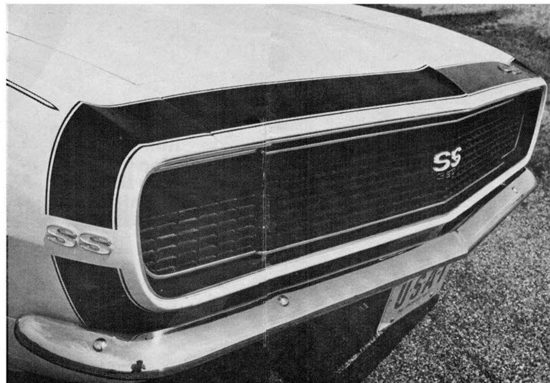
CAMARO SS 350 follows the well-developed pattern: Side and front letters identify it (stripe is optional), husky 350-cu. in. engine trimmed with chrome cleaner and valve covers powers it. This Camaro has retracting lights, too.
