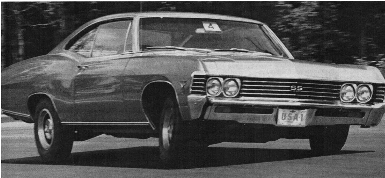
DADDY BEAR for the SS troupe is the Impala 427. Special front and rear grilles, big distinctive SS letters make it readily identified. The 427 engine package calls for firmer suspension, here being sampled by CL's crew.
