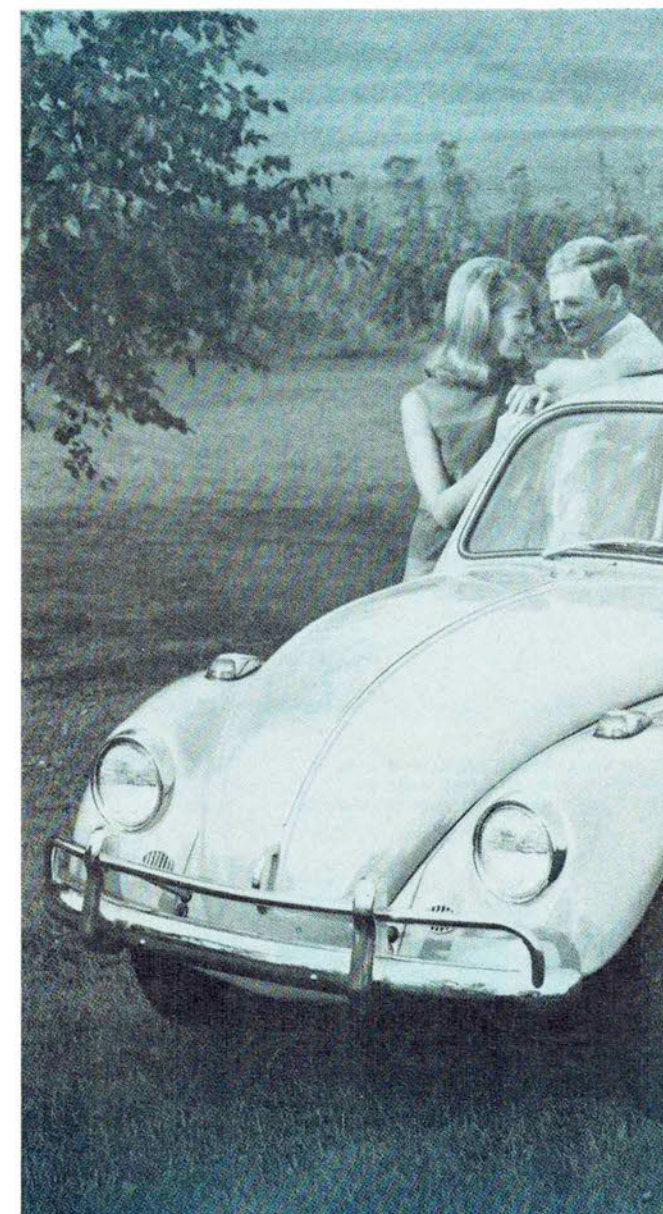
MAJOR EXTERIOR change, apparent in the 1967 VW is in front fenders, reshaped for more efficient headlamp mounting.
