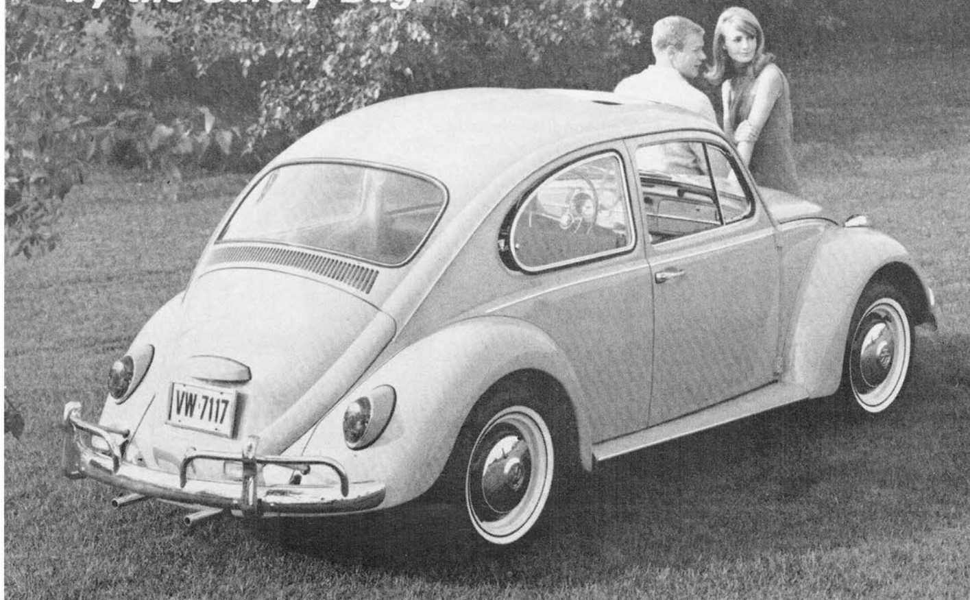
MUSCULAR NEW beetles are powered by 91.1-cu. in. engines, rated at 53 bhp—most powerful yet for VW sedans. U.S.-oriented safety items for '67 include tandem brake system, reversing lights, 2-speed windshield wipers and soft plastic control knobs.
