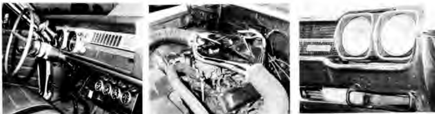
John Molnar lines up the Rund Olds for a blast down the Martin 131 Dragway tarmac. Best time to date is 111 mph in 12.40 secs. Hurst shifter with modified detents controls all-synchro four-speed. Rare factory-optional cold-air intake system tops off the Rochester tri-power intake system. Air intake is through front bumper vents. Setup is not listed for 1967 models.
