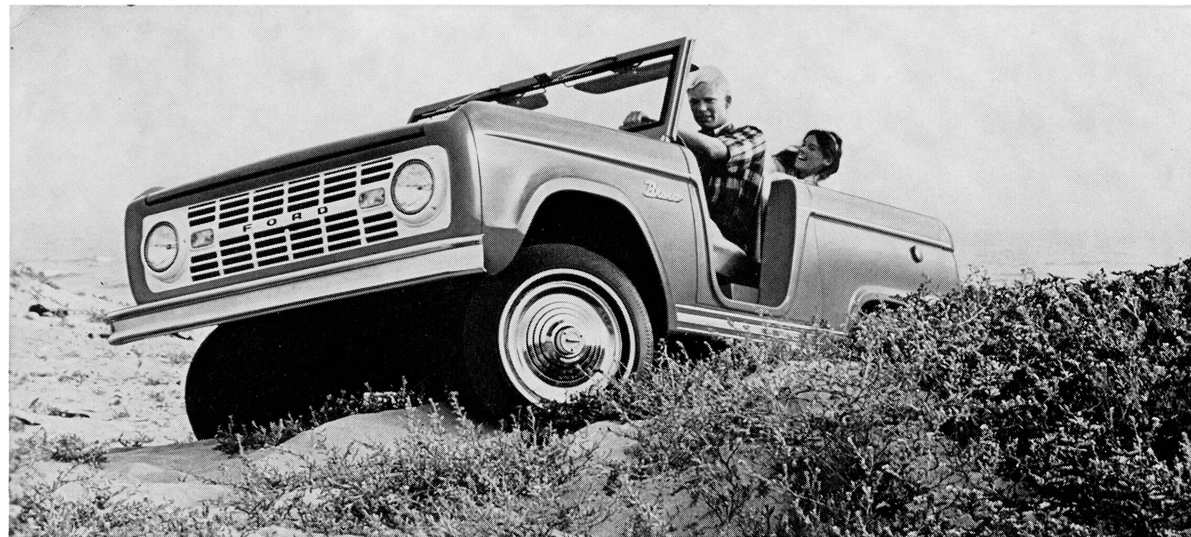
BRONCO ROADSTER ... Fun-loving open sports model with a windshield that can be folded flat and secured to hood. A convertible vinyl top with metal or vinyl doors is available. All Bronco models have 92-in. wheelbase, wide one-hand-operated tailgate, and big 14.5-gallon fuel tank.
