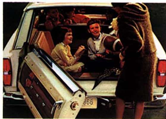
Now it's a door . . . for easier entry or close-up loading. New Magic Doorgate is shown on the '66 Ford Country Squire. Notice the dual-facing rear seats in this model.
