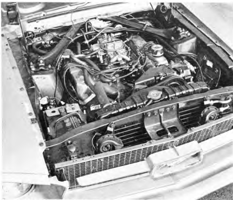
FORD'S PREMIER Ponycar is fitted with everything, up to and including the 390-cu. in./335-bhp engine.
