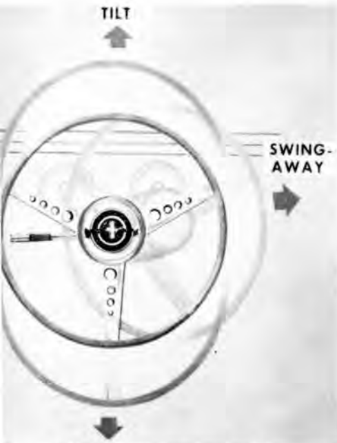
TILT/SWING column pops up and right for entry/exit ease, and has nine driving positions.
