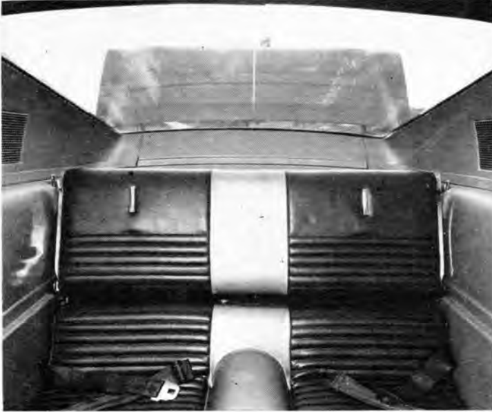
RAISED, THE upholstered underside of the rear deck panel provides a minimum of 2 plus 2 passenger accommodation.
