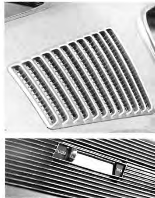
VENTS in rear roof pillar are operated from inside to provide straight-through ventilation.
