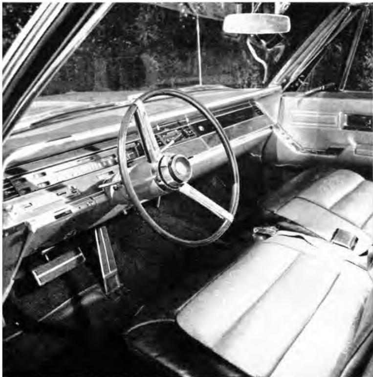
LUXURY-SAFETY interior was marred by highly reflective chromium plated mouldings at windshield perimeter.
