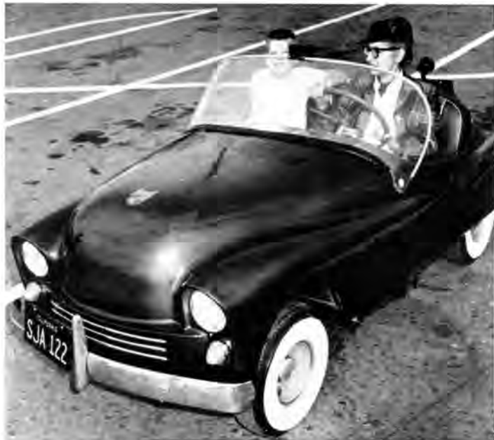
PRACTICAL battery-powered electric already is in use on Los Angeles streets. It has eight automobile batteries.
