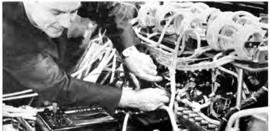
ELECTROVAIR II is second generation battery-powered car by General Motors Research. With a trunkful of batteries in front, and more batteries, the motor and controls (above) in the rear, the car weighs over 4000 lb. Range of the silver-zinc battery pack (value $25,000) is only 40-80 miles between recharges.
