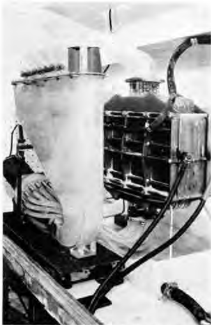
ZINC-AIR battery is one of the most sophisticated power sources under development, has an enormous potential for high energy density. General Atomic's experimental prototype model undergoes testing sequence, left. Cell stack is at right, zinc oxide separator in middle. Right, a schematic of the ZnO battery and necessary components.
