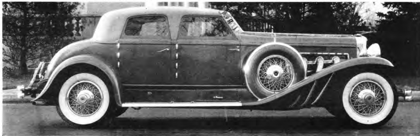
THE DUESENBERG Model J of the 1930s was priced at up to $20,000. Luxury and high performance were combined in this "Twenty Grand" model displayed at the 1933 Chicago World's Fair. A 265-bhp dohc engine produced speeds up to 110 mph.
