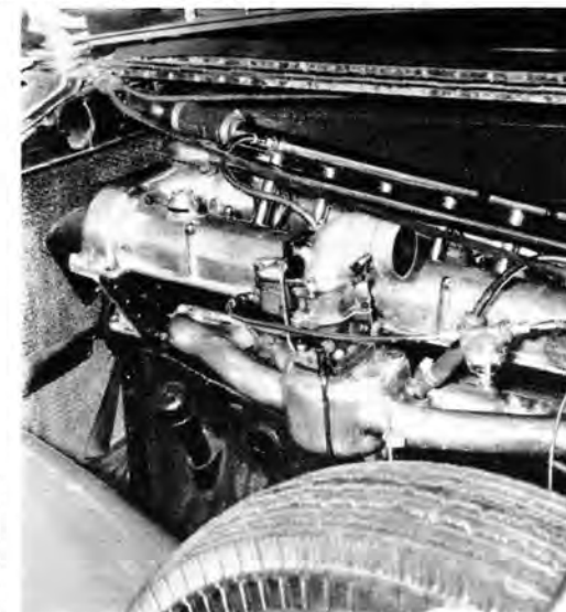
I N THE early 1930s, Stutz developed a 32-valve straight-Eight of 156 bhp, placed it in a short-wheelbase sports model. The car, manufactured in limited quantity, sold for $4600, was guaranteed to exceed 100 mph, and was named Super Bearcat.
