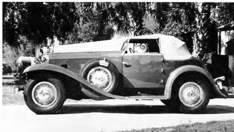
I N THE early 1930s, Stutz developed a 32-valve straight-Eight of 156 bhp, placed it in a short-wheelbase sports model. The car, manufactured in limited quantity, sold for $4600, was guaranteed to exceed 100 mph, and was named Super Bearcat.
