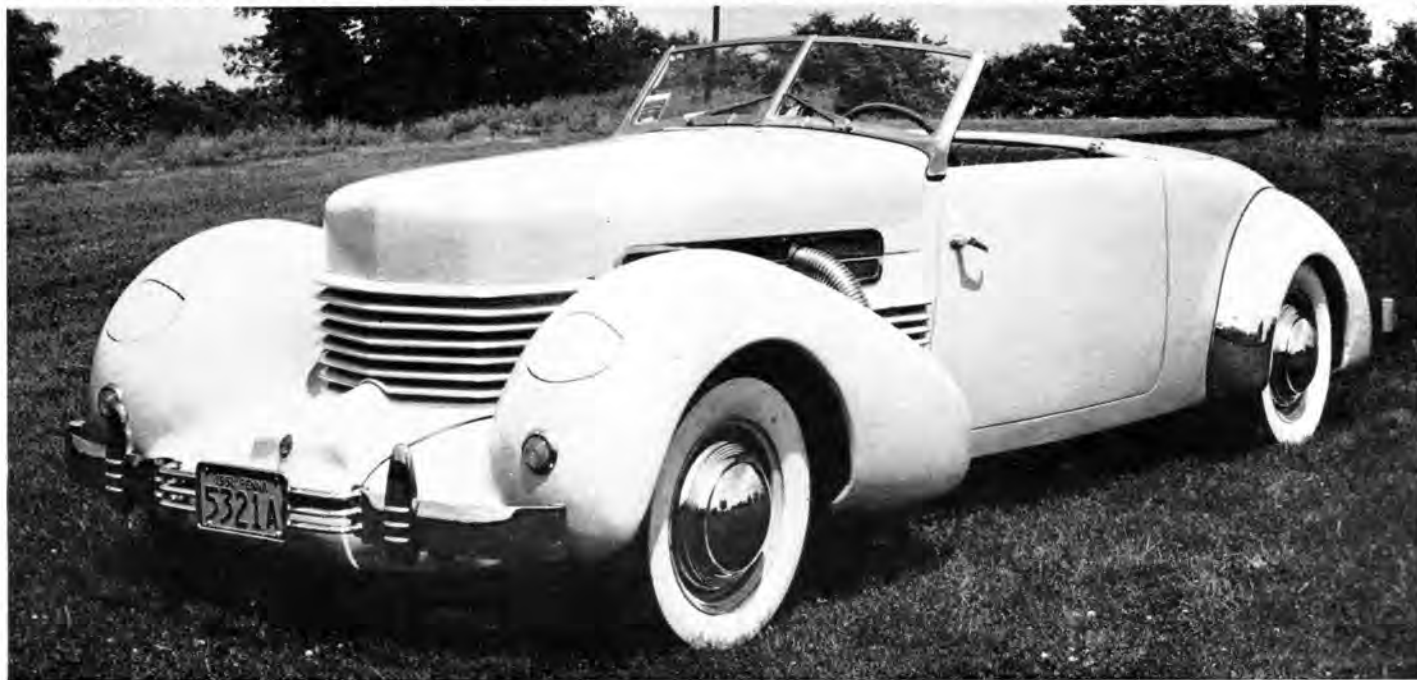
PERHAPS THE most famous of American high-performance cars, the supercharged 1937 Cord V-8 demonstrated exceptional handling qualities as well as 115-mph top speed and 0-60 time of 13 sec. This was a very large offering for a medium-priced car.
