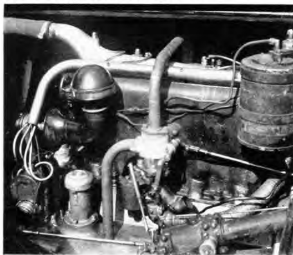
THE LARGE T-head engine delivered approximately 70 bhp at 2500 rpm for the Mercer Raceabout.
