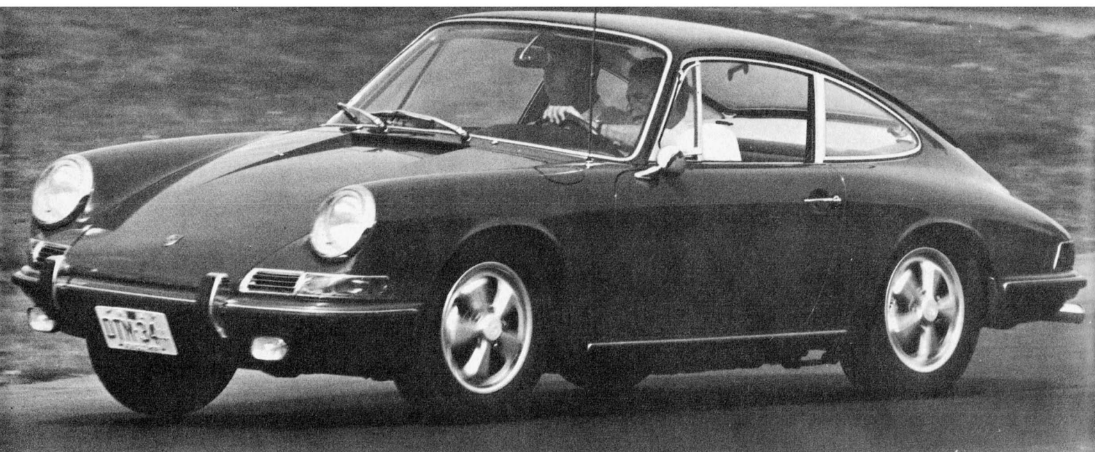
PORSCHE 911-S HAS LESS INITIAL UNDERSTEER THAN 911 OR 912, THANKS TO STABILIZER BAR, BUT TRANSITION TO OVERSTEER IS QUICKER.
