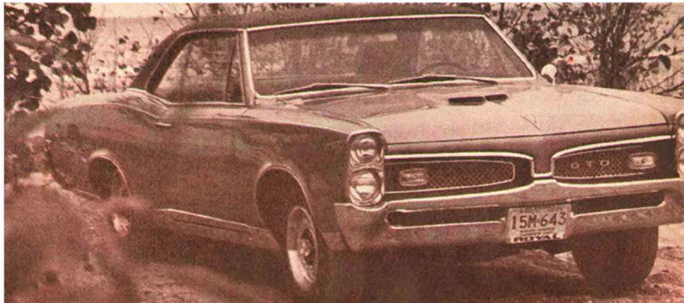
White test car had modified engine, hood-mounted tachometer, front disc brakes and Hurst wheels. Dark car retained stock engine with Rally I wheels, drum brakes.
