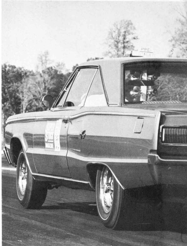
ABOVE —Although some of the pictures in this story show smoke coming from the stock tires, it was possible to bring the R/T off the line with a minimum of wheelspin. BELOW —Huge 440-cubic inch engine is the largest displacement engine offered in a high-performance automobile. R/T is also available with 426-cu. in. hemi, rated at 425-hp with two four-barrel carburetors.
