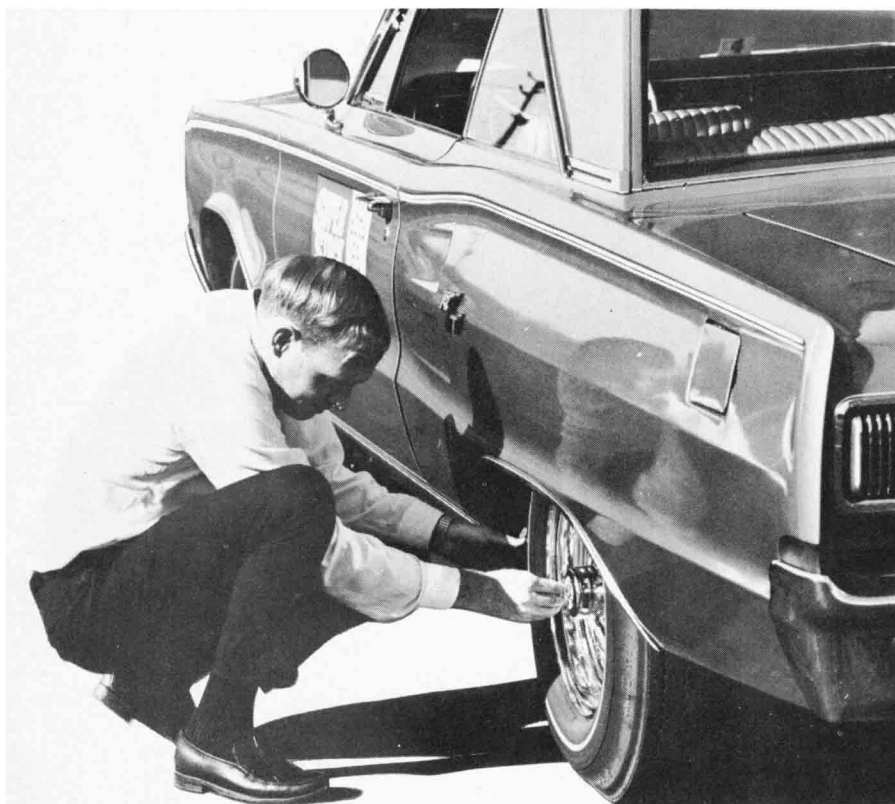
LEFT—Bill drops the air pressure a few pounds in an attempt to gain a few tenths of a second et. Varying the tire pressure didn't seem to help much as et stayed in the low 14-second range.
