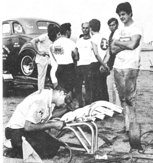
ABOVE—Jim Kerr of Hurst repairs a cracked header for Tom Ivo. That's Ivo in the Isky T-shirt talking to Marvin Schwartz. ABOVE RIGHT—George Hurst examines one of the many cars in the "hospital." RIGHT—Overall view of the Hurst facility.
