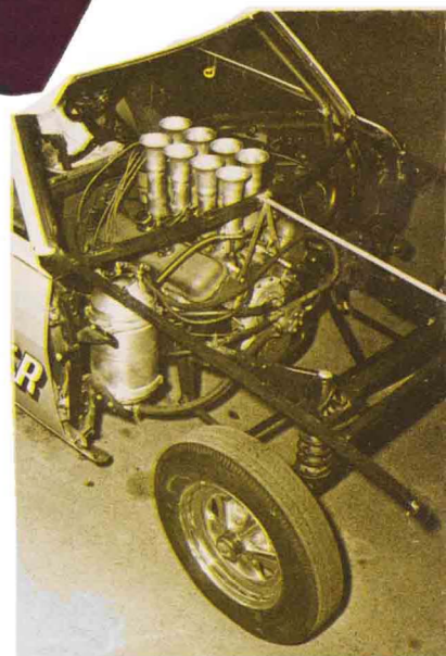
ABOVE — Smooth, aerodynamic front end of the '67 Corvair is conducive to high trap speeds. Slogan, "We Love Our Corvair," was inspired by auto critic Ralph Nader's remarks about overall Corvair design. LEFT—Driver, Del Heinelt, right, and mechanic John Ylitalo work on injected "semi-hemi" mill while Tom "Snake" Jones supervises. Entire fiberglass front end lifts off for easy access to fuel-guzzlin' engine. Note light, square-tube framework that extends from cowl to support glass front end. Straight tube front axle gets the job done with coil springs wrapped around Cure Ride shocks. Husky tube cage roll bar is also basis for chassis.
