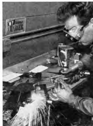
Frank Oglesby, who performed major portion of swap, prepares to remove jack from transmission after making crossmember modifications. RIGHT — Adding a new boxed section to center of cross-member, Oglesby found transmission would align perfectly with stock rubber pad.
