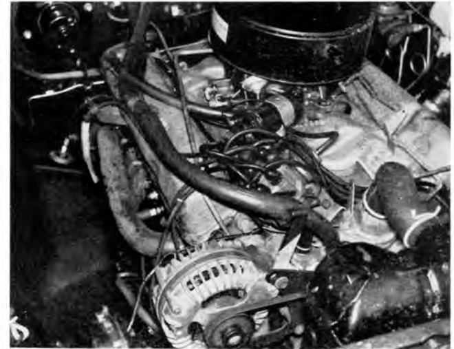
Closeness of the inner panels made use of stock exhaust manifold impossible without major cutting. Headers were answer.
