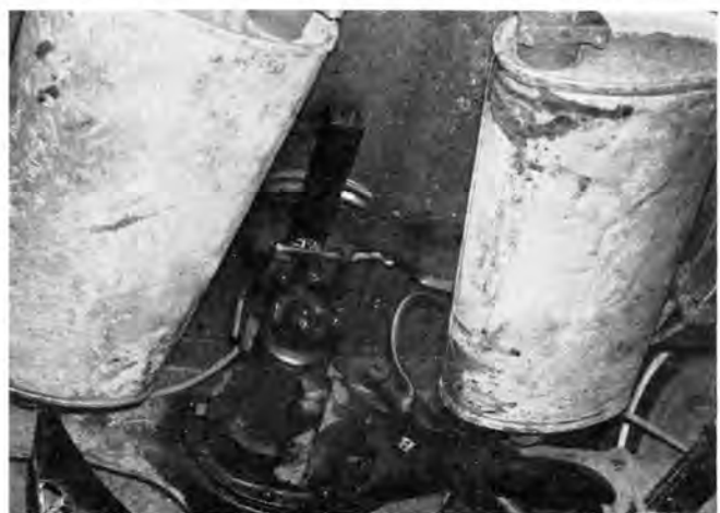
Extension was given pinion snubber in order to reach floor bracing. On acceleration car lifts eliminating axle wrap up.
