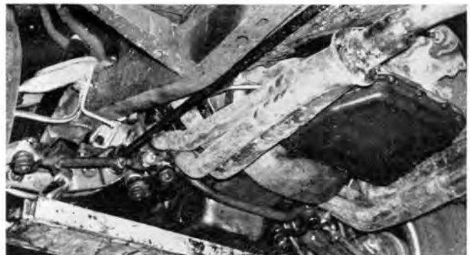
Iggy's custom headers had a tight fit weaving around steering and torsion bars. Shouldn't be a problem with factory casting.
