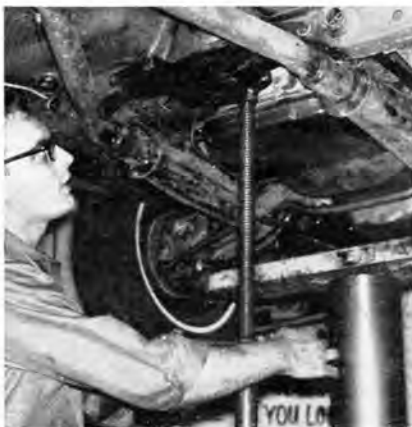
Frank Oglesby, who performed major portion of swap, prepares to remove jack from transmission after making crossmember modifications. RIGHT — Adding a new boxed section to center of cross-member, Oglesby found transmission would align perfectly with stock rubber pad.
