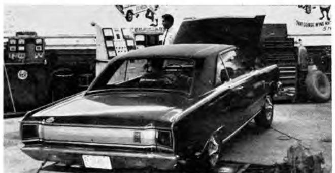
Leo Mattei and Oglesby check out the horsepower on Mr. Norm's chassis dynamometer. Read 390 compared to street hemi's 340.
