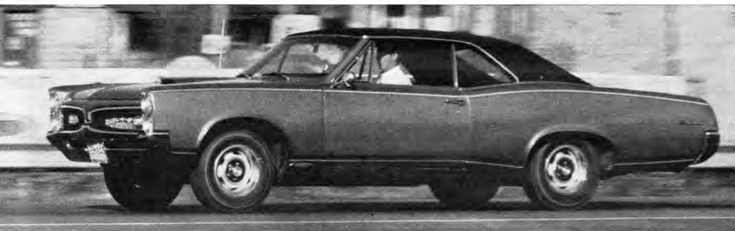
ABOVE —With Dave Warren driving, the showroom stock "blue" GTO turned steady times of low 14's at 100 mph. When the tires were changed to M&H slicks, times dropped into the high 13-second bracket.
