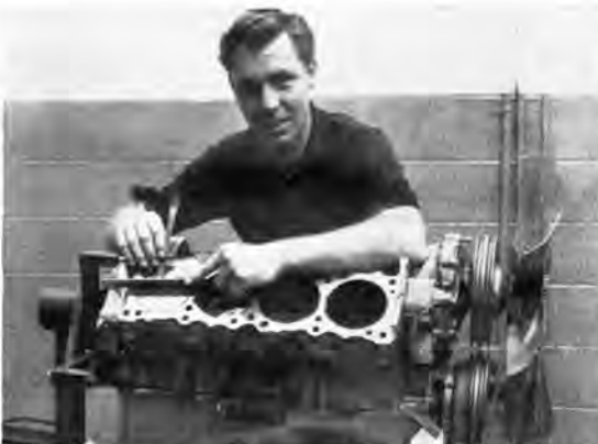
ABOVE — Sid Warren carefully measures the block deck clearance to the minimum .0015 during blue-priming of the engine. This attention to detail is where you pick up that additional horsepower needed to win.
