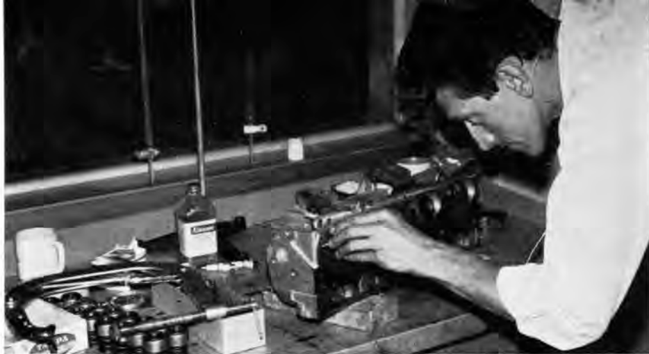
ABOVE —Milt Schornack, Royal's top drag racing expert, gives particular attention to the valve job during the Bobcat installation, saving time on the subsequent blue-priming operation phase of the program.
