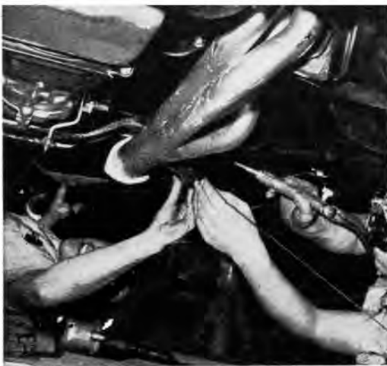
Bolting on a set of performance tuned headers is just like adding a few more horses. The white car came in for special attention with a set of Hurst experimental four-tube headers for maximum engine performance.
