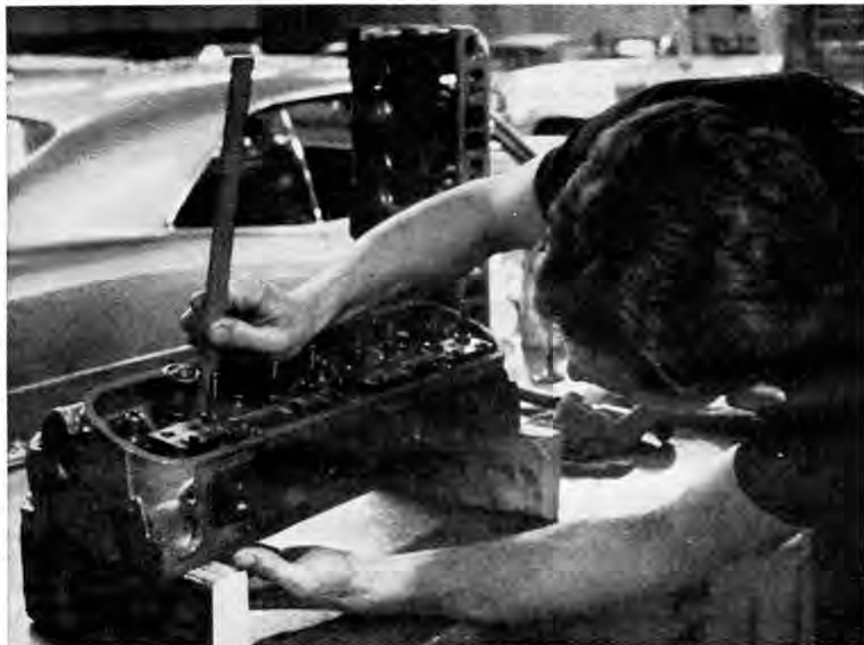
During the Bobcat phase of the testing program, the heads on the GTO came in for extra special attention in order to gain the additional engine speed necessary for shifts in the 6000 rpm range. Special sleeved lock nuts were installed as part of the Bobcat package, guaranteeing positive lash adjustment for thousands of street miles. A big gain in engine speed was realized by careful adjustment of the ball-joint rockers as outlined in the text in step-by-step style.
