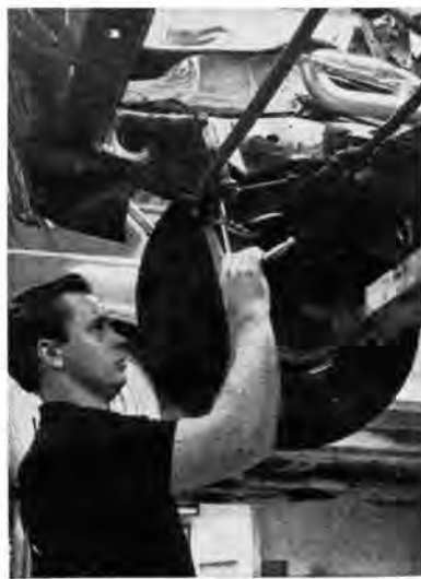
Extensive work was done to the front end on the blueprinted car, including installation of 90/10 Cure-Ride shocks for initial front end lift on hard runs.
