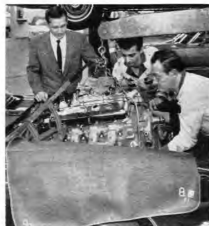
ABOVE LEFT — Mike Terrafino installs the big Holly on newly arrived 427 while "old" 350 awaits return to parts warehouse. No internal carb changes were made.
