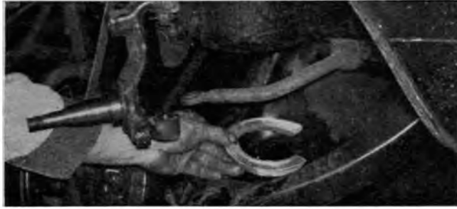
ABOVE — Additional 90 pounds of engine caused front of car to drop one inch. Air conditioner spacer is installed under the front coil springs to bring the Camaro back to the stock height. RIGHT — Harrell modifies the single point 427 distributor by installing heavy duty points with their greater spring tension. Advance curve is adjusted for each car's specific use.
