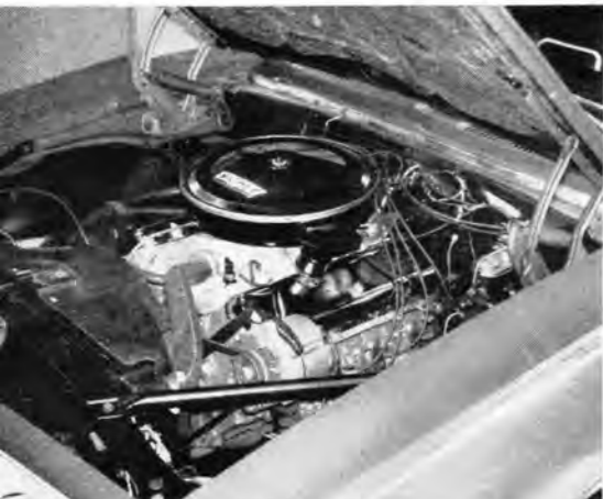
LEFT ABOVE — Until Nickey made their 427 Camaro available, the 350 cubic incher was Camaro's biggest engine option. Based on the 283 block, the 350 left a lot of space for changes.
