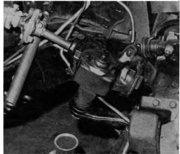
ABOVE—Chevy II traction bars are stocked by speed shops and are a must on the Camaro. The lower unit was converted by shifting the shock mounting bolt. LEFT — Number five exhaust manifold header is the only engine component to feel the grinder. Heavy casting easily gives up 1/16th-inch with no ill effects. RIGHT — Steering box gets corresponding "narrowing" by having its upper right corner ground to 45 degrees. That's all that is needed to stop the rattles.
