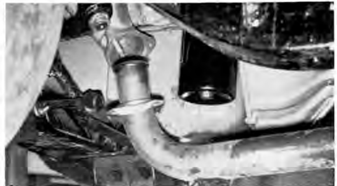
The 427 exhaust manifold and 350 head pipe have nothing in common, meaning the head pipe must go. Clearance around bottom of engine leaves lots of space for steering linkage to move.
