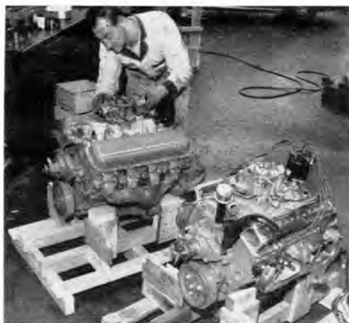
LEFT ABOVE — Until Nickey made their 427 Camaro available, the 350 cubic incher was Camaro's biggest engine option. Based on the 283 block, the 350 left a lot of space for changes.
