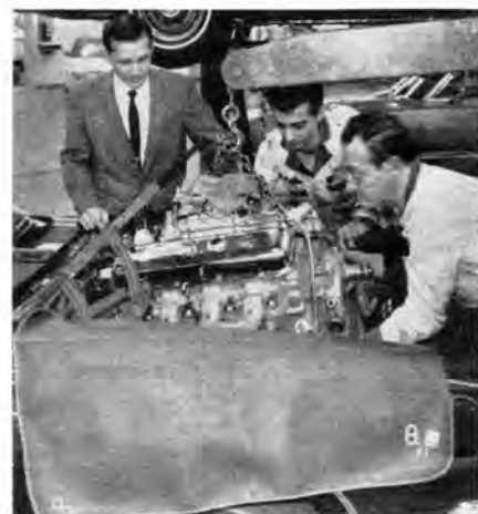
ABOVE LEFT — Mike Terrafino installs the big Holly on newly arrived 427 while "old" 350 awaits return to parts warehouse. No internal carb changes were made.
