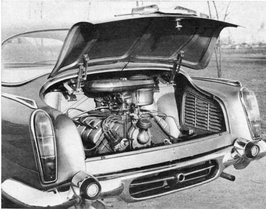
CZECHOSLOVAKIA'S TATRA luxury model retails for $2550 in the West, but sells for $22,500 to Czechs. Power is from a rear-mounted, air-cooled V-8.
