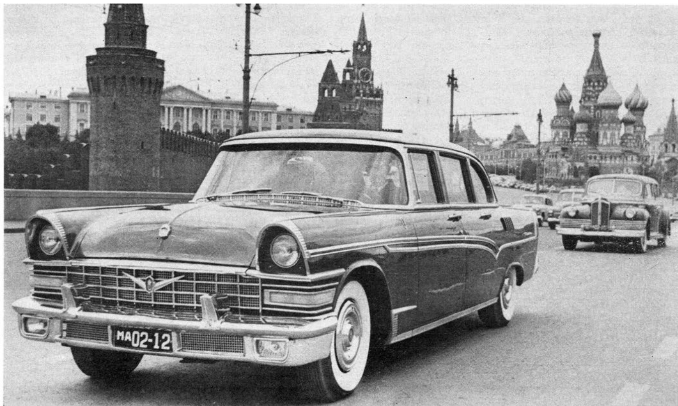
THE PORTLY ZIL-111 , in 1958, was Russia's automotive answer to the West. Automatic transmission, power brakes and steering, windshield washer, tubeless tires, power windows, radio and 105-mph top speed were touted. Few cars were built.
