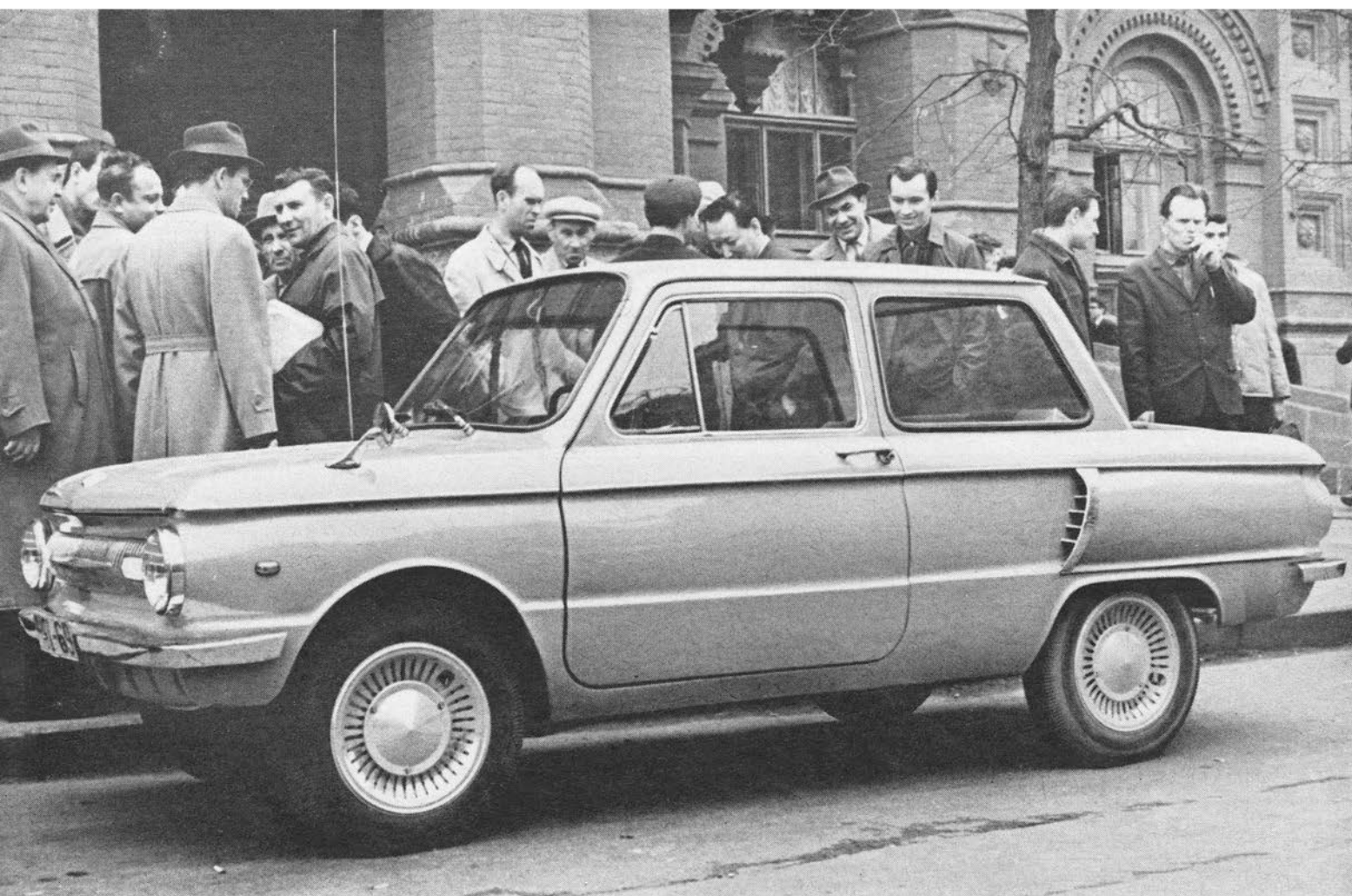
THE RUSSIAN Zaporozhets ZAZ-966 was put into production in 1966. The car now is powered by a 4-cyl., 27-bhp air-cooled engine, but a 40-bhp unit of the same type is being readied for future installation. At the rear, Muscovites admire the new model.
