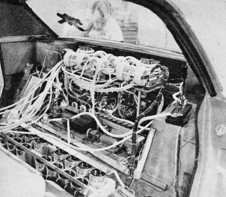
COILS, CAPACITORS and switches form the control system for Electrovairster II—and completely fill rear seat area.
