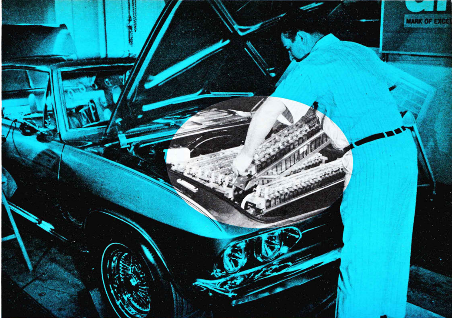
A TECHNICIAN loads silver-zinc batteries into the forward compartment of the Electrovair II preparatory to a test on the chassis dynamometer at General Motors Technical Center, Warren, Mich.
