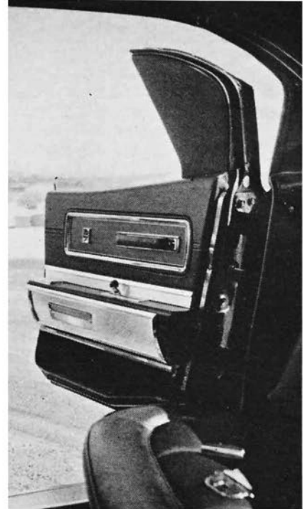
PART OF the rear roof pillar swings out with the door to give a broader opening.
