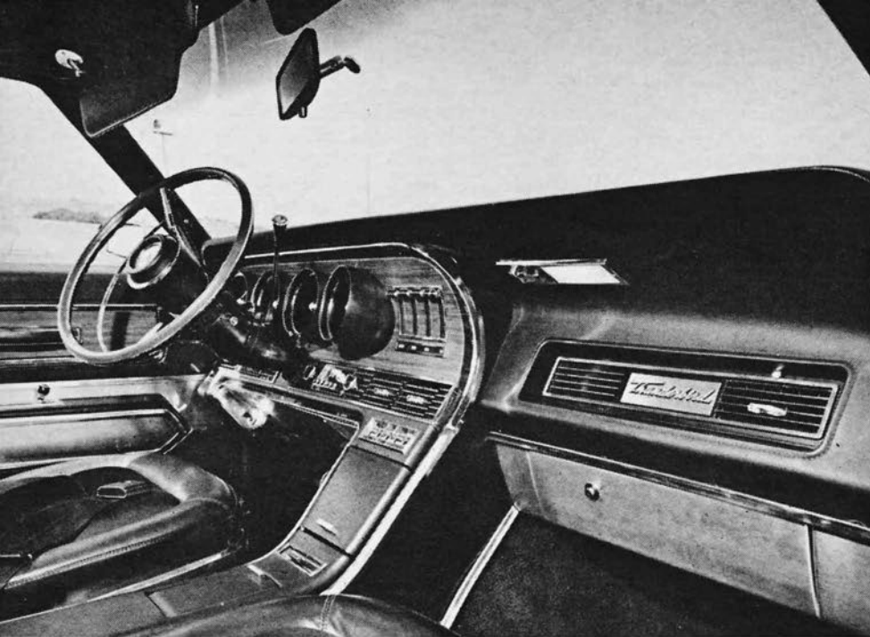
THUNDERBIRD'S "flight deck" shows abundant use of chrome plating, simulated wood texture, vinyl covering and projecting instruments, knobs and levers.
