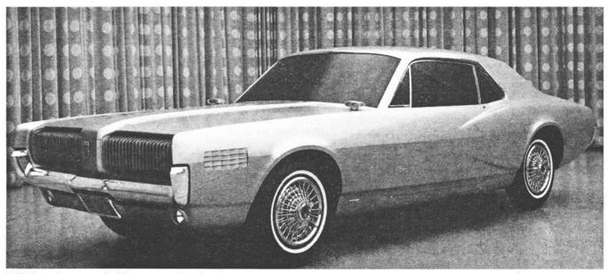
AS THE deadline approached for approval of the final Cougar design, groups of designers prepared clay models for a selection showing. The model above introduced the divided wrapover grille treatment, with vertical lines and concealed headlamps which are retained on production Cougars. Rear fender elliptical lines have disappeared, however.
