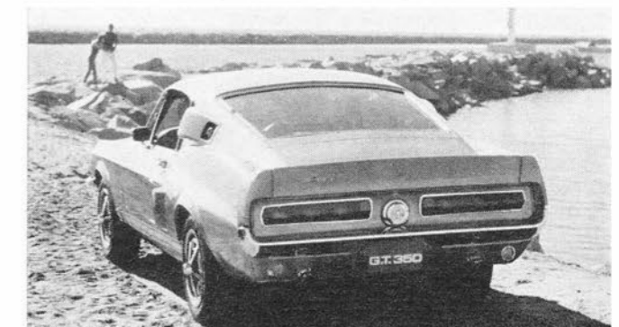
SCOOPS AND a spoiler tail, for a husky horizontal look, mark the 1967 Shelby Mustang GT 350. Rollover bars that meet competition specifications and inertia reel shoulder harness for drivers and passengers are fitted. Gearbox choice is between 4-speed manual and 3-speed automatic.
