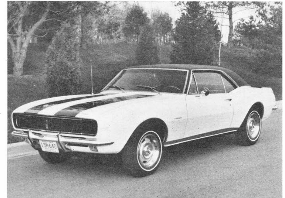
ROADWORTHY CAMARO with the latest, Z-28, option package is suitable for all kinds of fun and games. Engine has 302-cu. in. displacement (283 V-8 stroke with 327 bore) and big-valve heads, solid lifters, huge Holley 4-barrel, tuned headers and special ignition. Suspension is all heavy duty and disc front brakes are standard. The 4-speed manual transmission has the 2.2:1-first gearset and final drive is 3.73:1 (but 3.07 to 4.88:1 are available). Dual paint stripes and rear deck lip "spoiler" make it a visual as well as performance standout.
