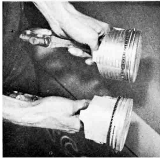
Right, stock 389 slugs must be notched to conform to 400-type heads.
