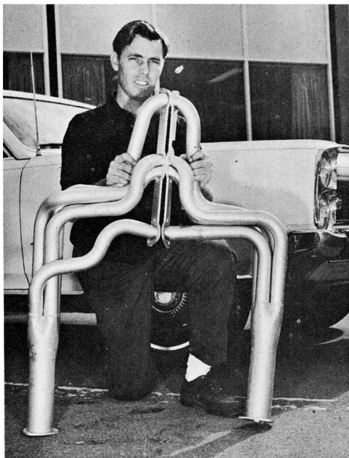
Above left, new 400 headers will fit all past 389's. Right, better top-end punch is achieved by blocking heat riser passages.
