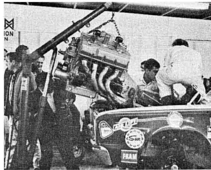
Chrysler hemi has specially-designed con rods for long-track endurance.
