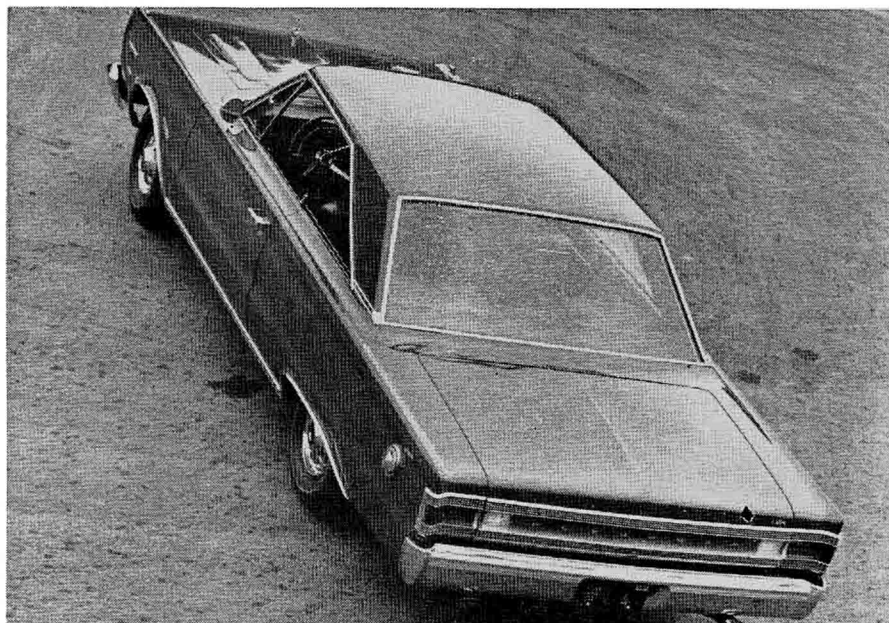
Wide rear window, thin "C-post" allow drivers to see rear non-fin tender tips.
