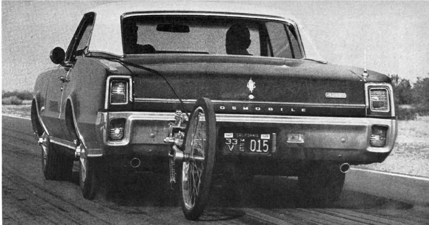
4-4-2 is able to get even, positive bite with smooth Anti-Spin differential, allowing duplication of times within small spread.
