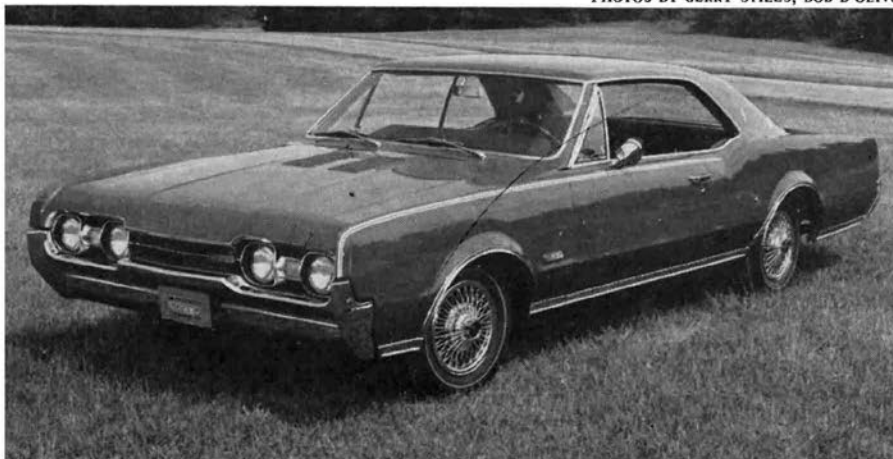
Simulated wire wheel covers on 4-4-2 do best job of cooling optional front disc brakes.
