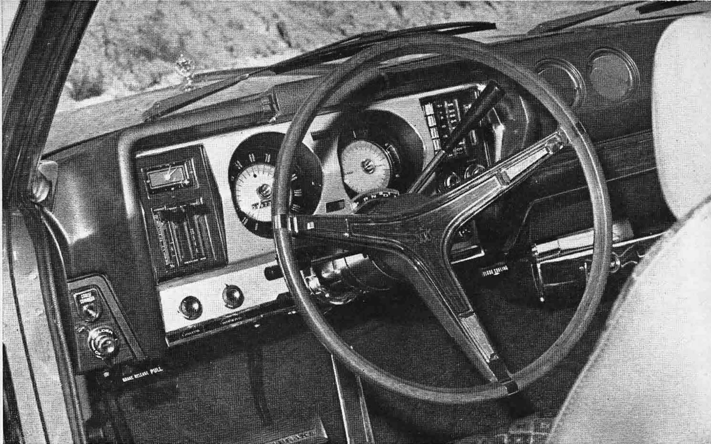
DPL instruments are well lit and easy to read. Speedometer is marked every 1 mph. Idiot lights remain for amps and oil.
