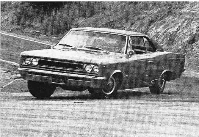
"Wash-out" tendency of SST is revealed on hard corners, but normal use shows front suspension strong, stable and firm.
