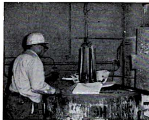
A few camshafts, along with some metal rods are about to receive the case hardening at E&J Heat Treating in L.A. That furnace is filled with a liquid cyanide, and carbon from the cyanide is absorbed by the surface of the heated camshafts, resulting in a harder surface for better wear. Copper plating certain areas prevents hardening.
