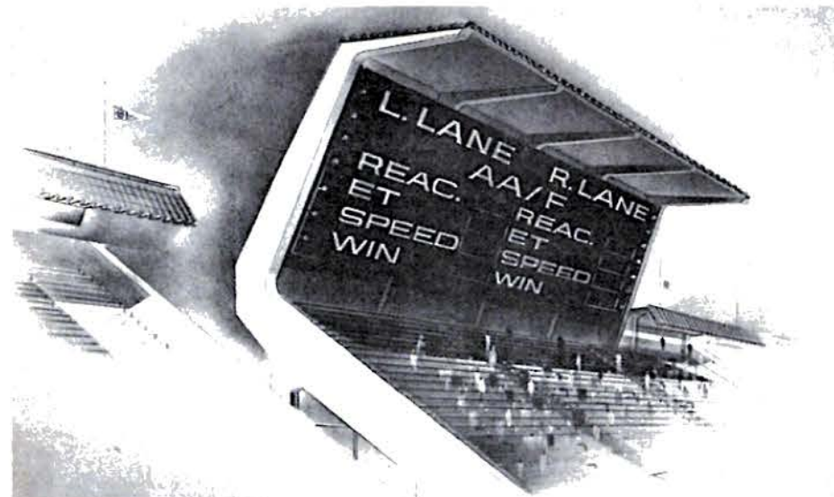
Grandstand mounted electronic scoreboard is tied directly into Christmas tree starting system. Elapsed times and speeds for both lanes are instantly recorded in lights.
