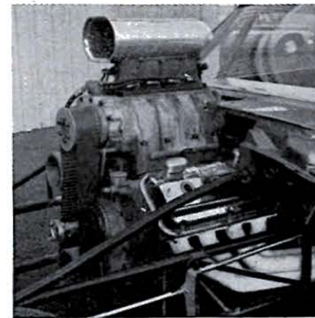
The heart of it all is the supercharged Chrysler of gargantuan dimensions. Big 448-inch hemi feeds on alcohol mixture.
