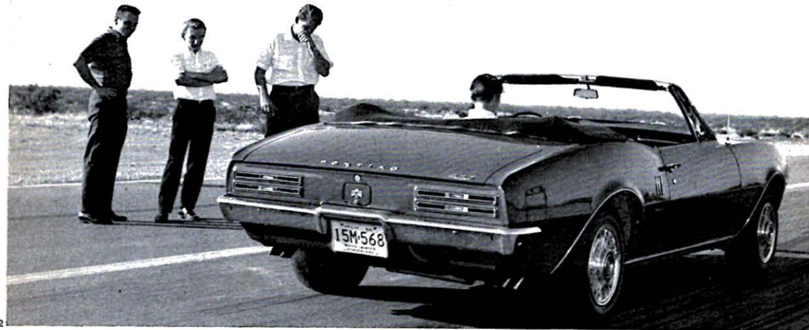
1 The Firebird is the first of the fun cars to combine grille and bumper into one unit providing an uncluttered look. Headlights mount horizontal rather than vertical as on the other 1967 Pontiac models.
