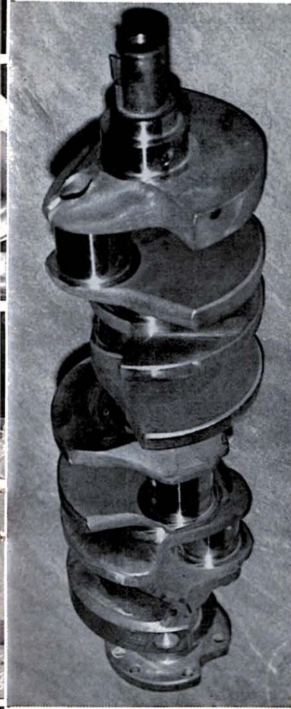
LEFT — Another "must" in the good engine was a Crankshaft Co. product, although 283" stocker unit worked very well in the first engine. Components can be added separately as you go along.
