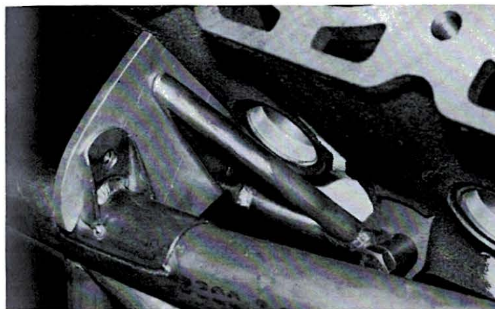
A close look at the front motor mounts shows where a small plate was welded on the frame rail to spread the stress, a bolt hole indicates solid mounting, and clever tubular brace to the engine block.
