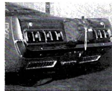
Wait until you see those T-bird lights blink sequentially during the burnouts. Corvair vents below bumper allow air to escape from body, filling Simpson chute.
