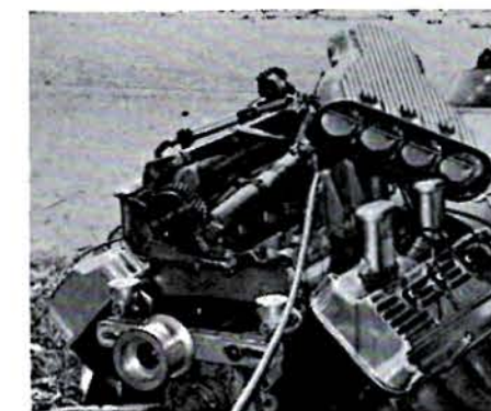
Violent force from blower explosion hurls parts and pieces over a wide area. Cover would hold pieces and help choke fire.
