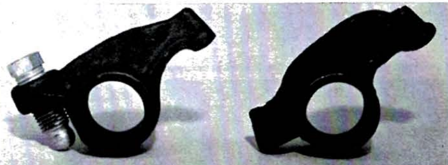
If you have hydraulic lifters in your Ford, chances are the engine has non-adjustable rocker arms like the one on the right. The one on the left permits setting the valves.
