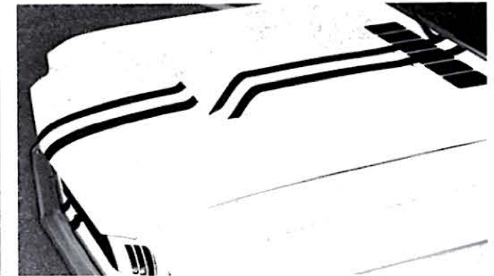
Ford's "J" prototype sports car motivated the development of this unique hood design which eliminates all lift and heat.
