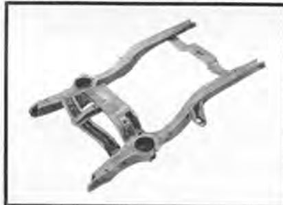
FRONT sub-frame carries suspension and engine/transmission in rubberized isolation.
