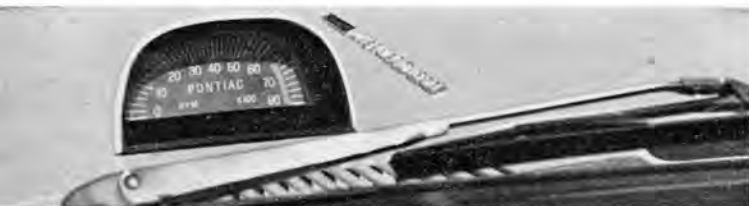
HOOD-MOUNTED tachometer is a feature of the sohc Six Firebird, as is the "overhead cam" lettering alongside the hood bulge.
