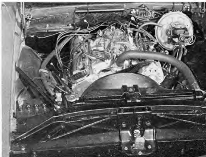
BIG V-8 supplies plenty of muscle for Firebird flight. Fitted with 4-barrel carburetor, 10.75:1 compression, it beats out 318 bhp.
