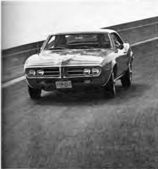
LONGER FRONT overhang gives Firebird 188.4-in. overall length, though it shares 108.1-in. wheelbase of 3.8-in. shorter Chevrolet Camaro.
