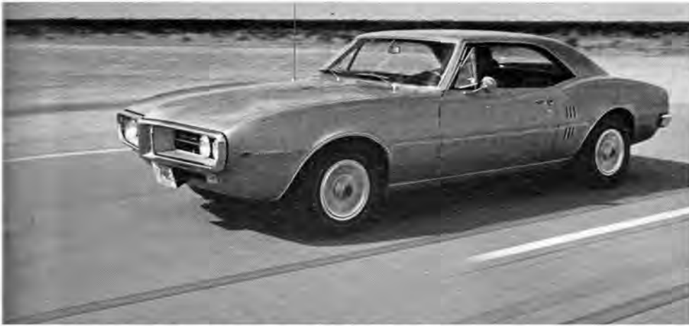
LONGER FRONT overhang gives Firebird 188.4-in. overall length, though it shares 108.1-in. wheelbase of 3.8-in. shorter Chevrolet Camaro.
