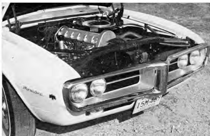
HIGH-WINDING ohc 6-cyl. engine barely fits under low hoodline but is an admirable performer in the lighter-weight Firebird chassis.
