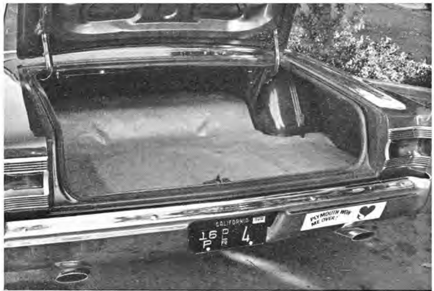
PLYMOUTH CREATES a broad, flat trunk area by placing spare tire in a well below the floor. Fuel tank fills from side panel, also fits under trunk floor.
