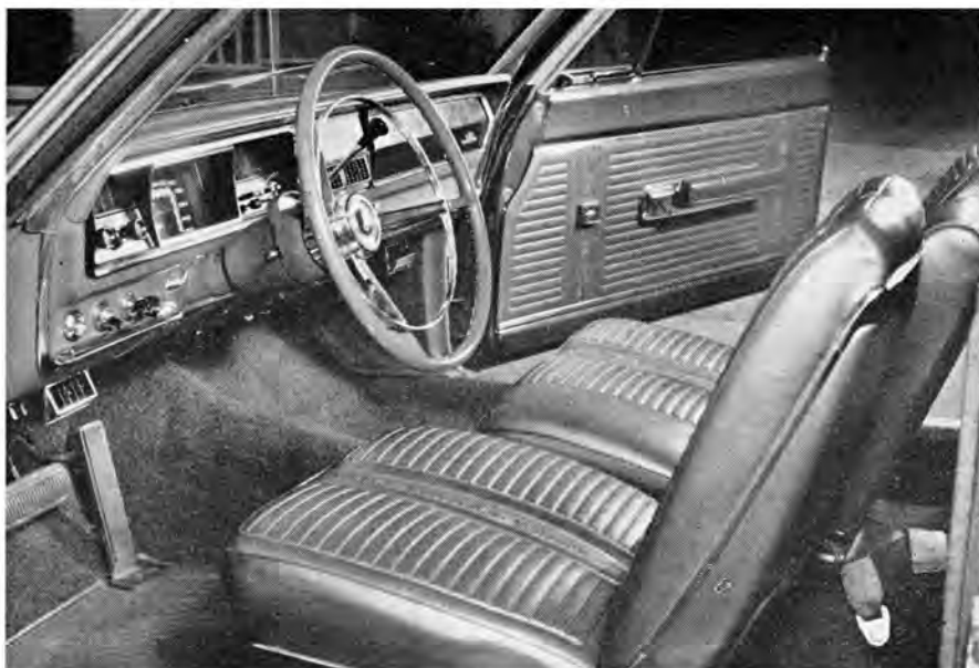
BUCKET SEAT interior is all-vinyl finished, with heavily embossed seats and panels. Automatic transmission shift lever is up on column, leaving floor area clear.
