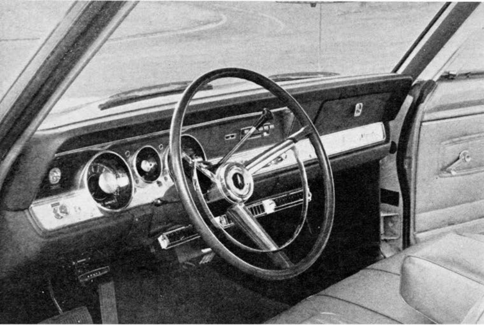
HARDTOP SIX interior featured bench seat with fold-down armrest, column shift, extra-cost vacuum gauge and under-dash air conditioner outlets.
