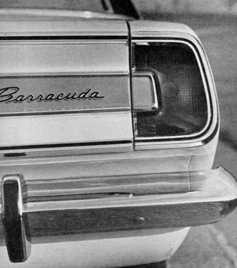
AMBER RUNNING lamps, switched on with headlights, flip top filler cap are Barracuda trademarks. Adequate trunk space, vulnerable filler pipe arrive with the hardtop.
