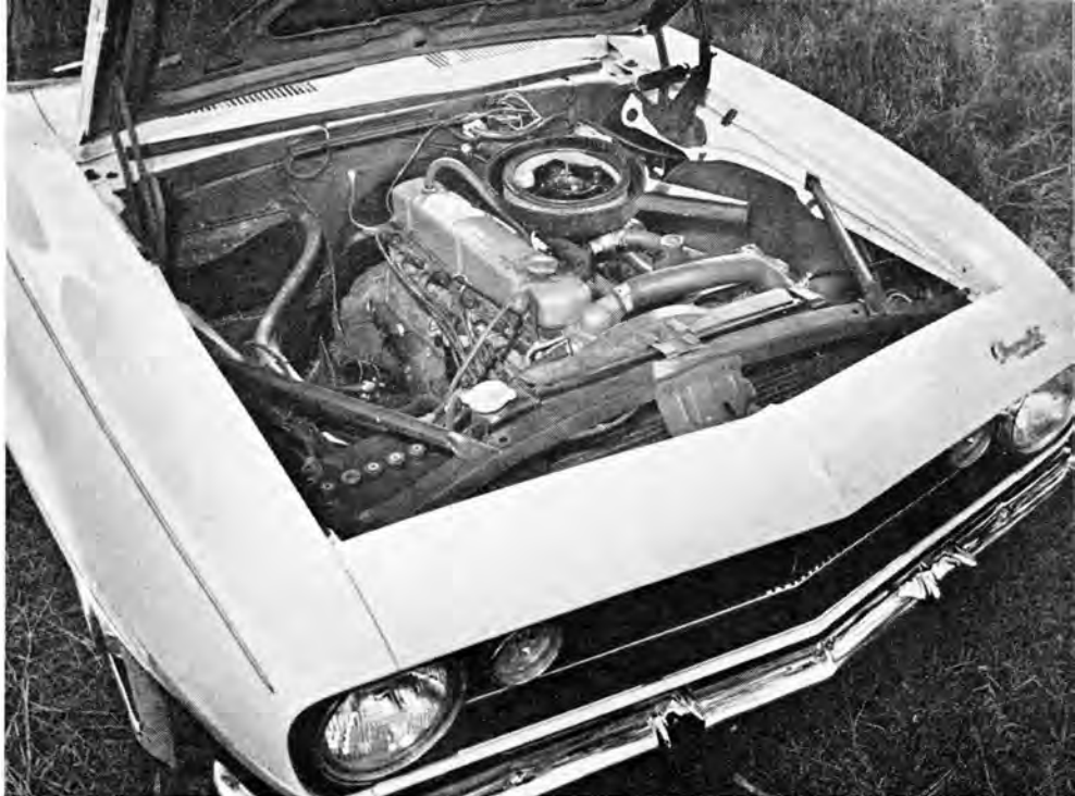
BIG SIX engine takes up less space, has greater access for servicing. Performance of this engine is surprisingly good for only 250 cu. in.
