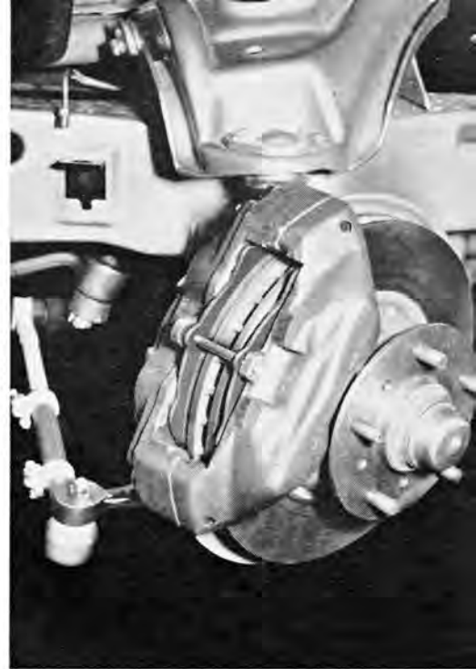
DISC brake option uses radially-vented rotors and four pistons per caliper.
