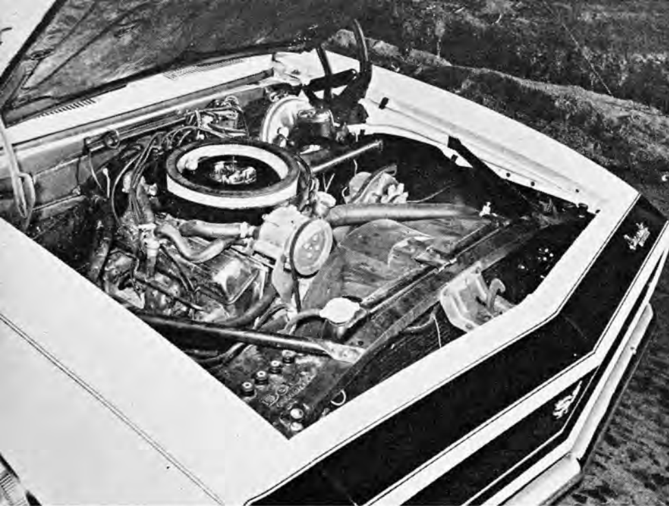
ENGINE COMPARTMENT of SS 350 is filled by engine, though there's enough space left for power accessories, air conditioning.
