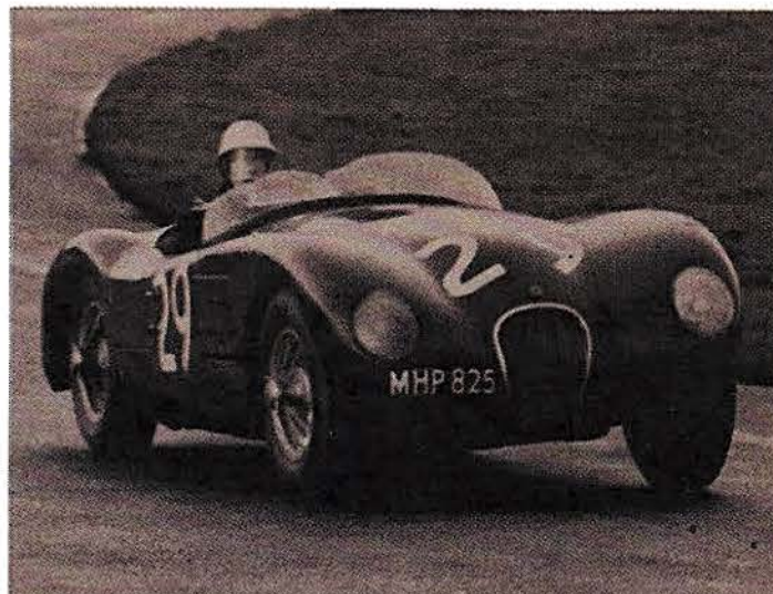
The C-Type Jaguar had classic nose design for proper air-guidance over it.
