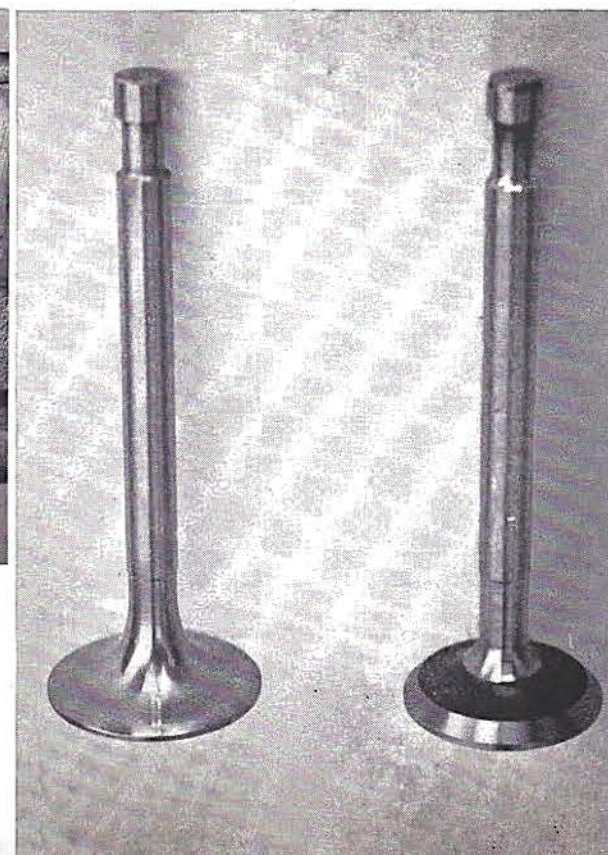
At left, a fully prepared head, with polished and lightened valves, relieved combustion chambers, etc., is a thing of beauty. Right, most of the rework is concentrated on the intake valve since the gas flow is from beneath the head and heat is less. A proper porting job, above, provides unrestricted flow, is most critical in the guide area.
