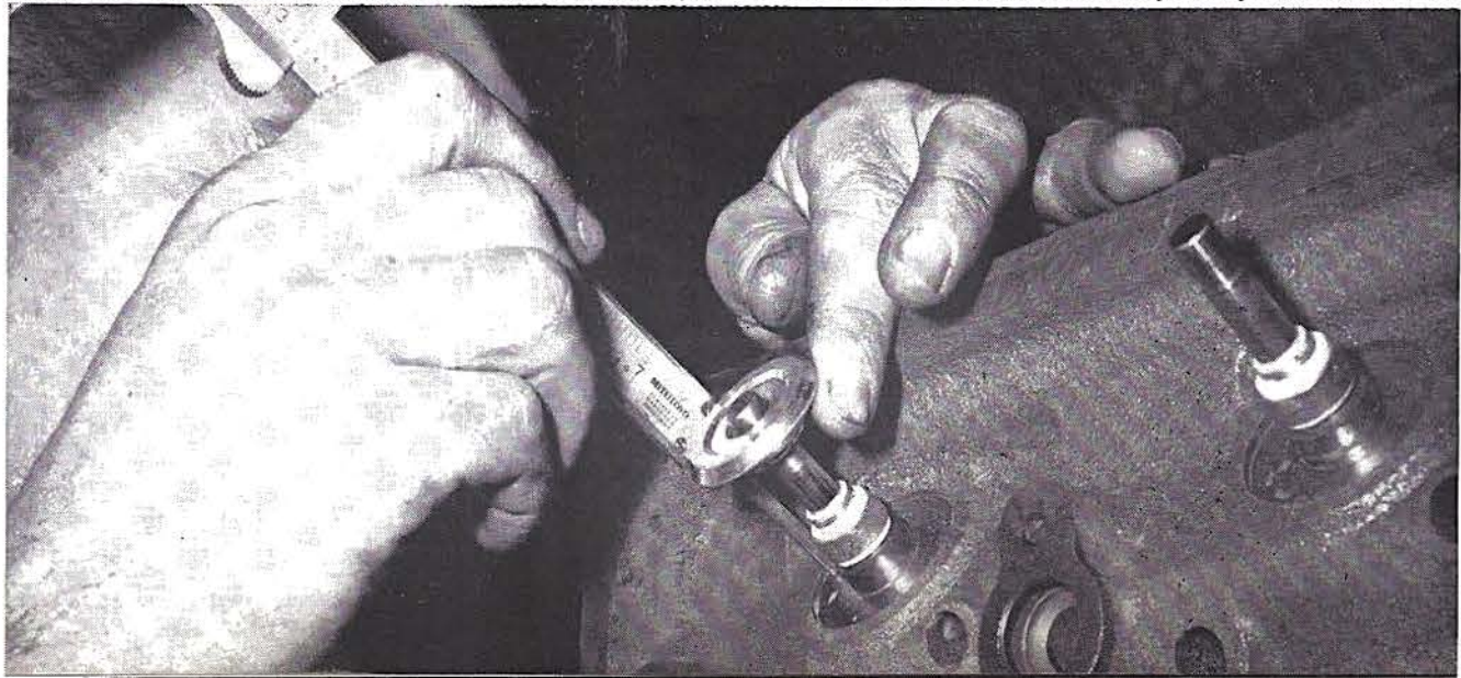
Total spring height with the valve in closed position is critical for equal pressure. Shims or sometimes grinding of the spring seats is necessary to get desired height. A hemi head is shown here, with intakes in line. Perfect Circle seals have already been placed in valve stems.
