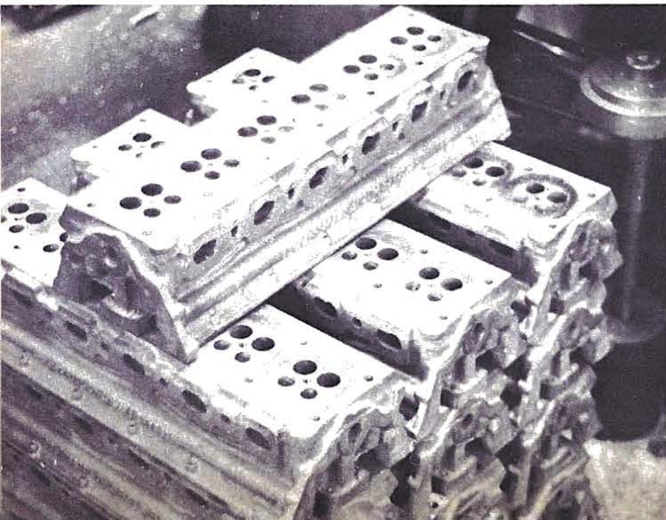
An expensive pile of cordwood! Cylinder-head castings are stacked prior to machining. The junction of exhaust ports for each cylinder is cast into the head, but intakes separate.
