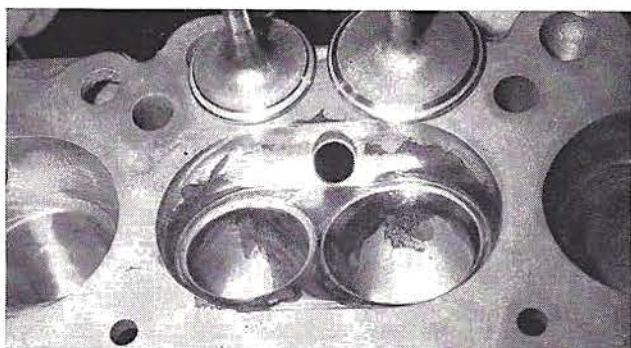
A pre-assembly check with machinist bluing after a light hand-lap of the seats shows the ideal widths to accomplish for intake and exhausts.
