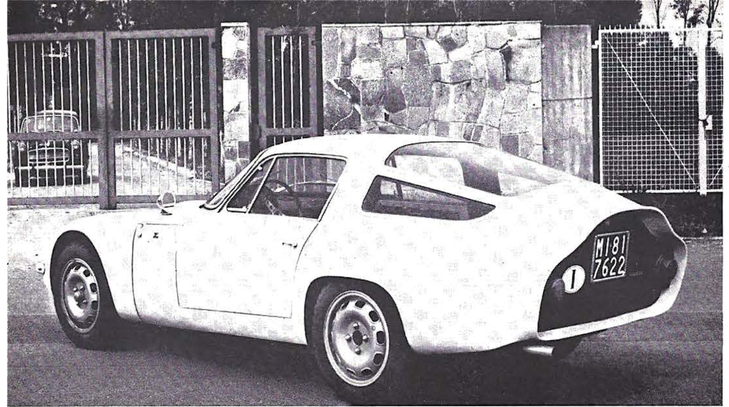
An almost classic example of the Kamm theory (chopping a mathematically tapered tail at a specific point) is the slippery Alfa Romeo GTZ.
