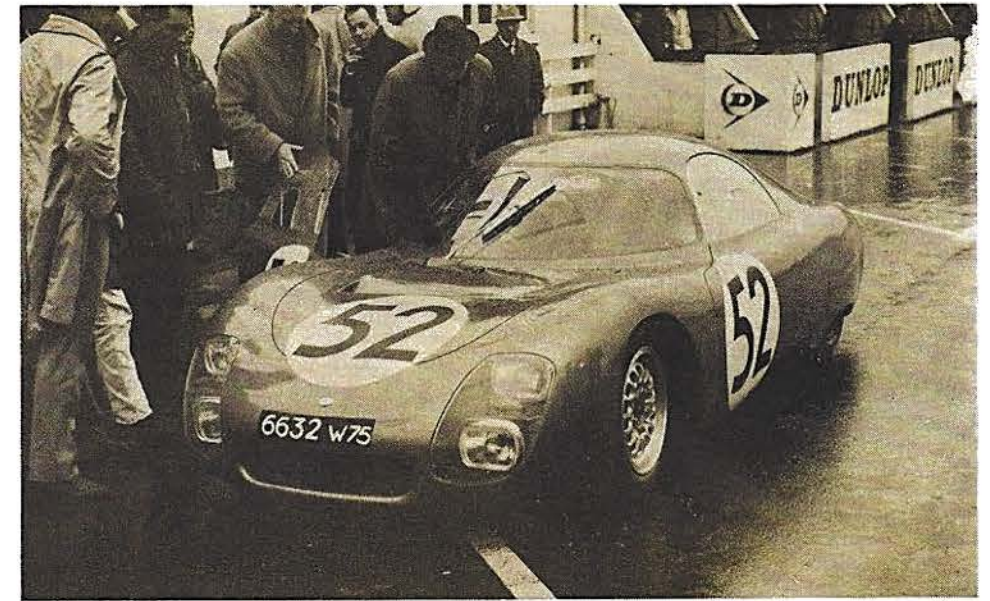
The LeMans CD Peugeot, at right, and the McLaren at left, both show attention to airflow over the nose and in grille openings. The Peugeot is more refined in this respect, but its design restrictions are not as limited.
