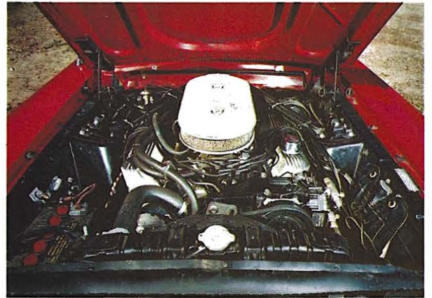
The powerful GT500 (instrumentation and engine compartment shown at right) uses two four-barrel carburetors atop the 428-inch engine. Our test unit was equipped with air conditioning and automatic transmission. The sparkling GT350 shown in photos below makes good use of the wider track for improved ride and superior handling in tighter corners.
