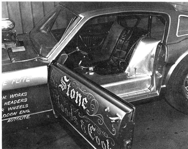
ABOVE—1967 T-Bird taillights grace rear of car. Special body work was performed by Ronnie Olson. Tri-form chute is by Simpson. Note 11-inch wide M&H drag slicks. RIGHT—Another view of the super custom interior. Although the basic body shell is steel, the hood, fenders and doors are fiberglass, contribute to overall low weight of only 1200 pounds.
