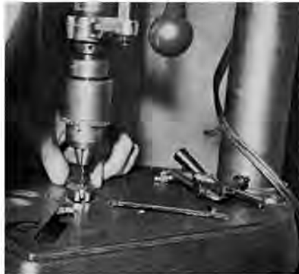
The primary jets were opened up .002 inches to improve mid-range response.
