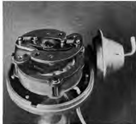
Advance curve of pointless sparker was quickened using Chevy springs.
