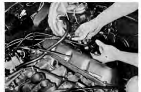
Hole left after removal of PCV gear was fitted with a right-side breather.
