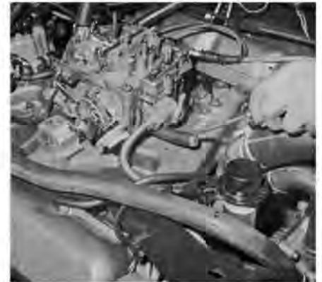
PCV "garbage" was done away with and the line to the quad blocked.
