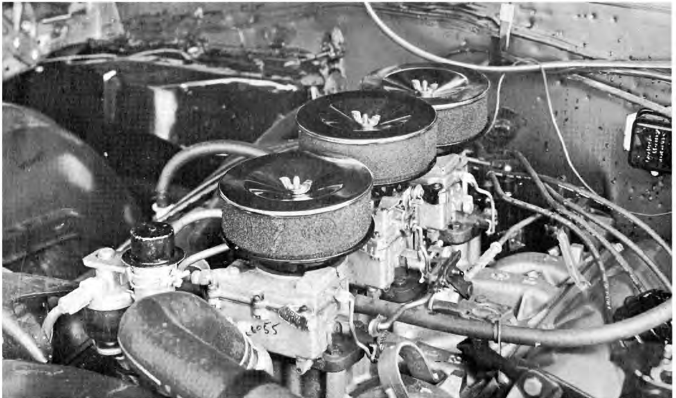
Factory tri-pot manifold and W-30 Cold Air kit are factory available on a do-it-yourself basis. It's the hot setup!
