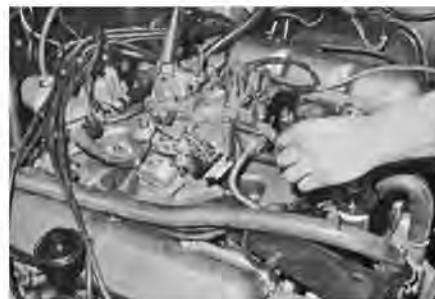
After the 35-degree advance curve was plotted, the vacuum takeoff was plugged.
