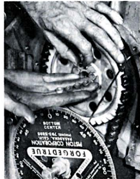
ABOVE—Every one of the valve springs should be assembled to the same height for maximum engine efficiency. Here a technician measures height of one spring assembly before adding shims. Spring seat cutting requires a special tool. BELOW—The correct phasing of the camshaft to the crankshaft is also important to obtaining maximum power from a given engine. The cam can be put in stock phase, and it can be either retarded or advanced from stock phase by machining the cam gear to receive special offset bushings or "cam keys." The gear must be machined according to instructions to get the best results.
