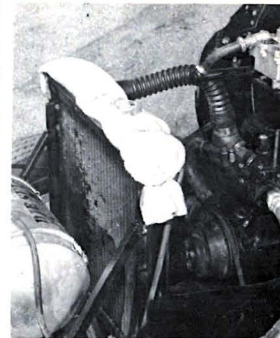
ABOVE—The Fenner Tubbs Plymouth is fitted with a zippered canvas bag that holds ice. When the ice melts, it passes through the fiber and trickles down across the entire radiator face. Then the water evaporates and carries off heat from the radiator. ABOVE RIGHT—Another idea for efficient cooling is hosing down the radiator face and keeping a towel on the top tank to hold water, release it during a run. This gasser runs without a fan, so other methods are needed. BELOW—Hood modifications, where allowed, will help. Holes in rear let hot air get out.
