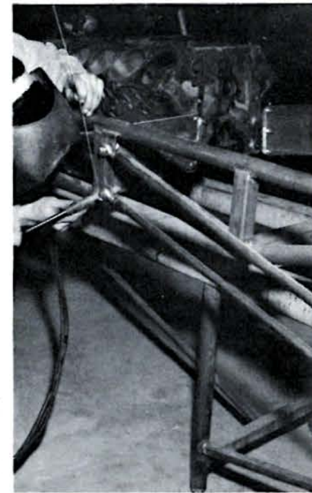
ABOVE —George Britting checks out the view from the bridge of a Dodge Charger funny. Cage protects driver in the event of a roll, and cut out area provides working room. RIGHT —Chassis technician uses heliarc welder on radius rod mounting bracket to provide strongest joint possible.
