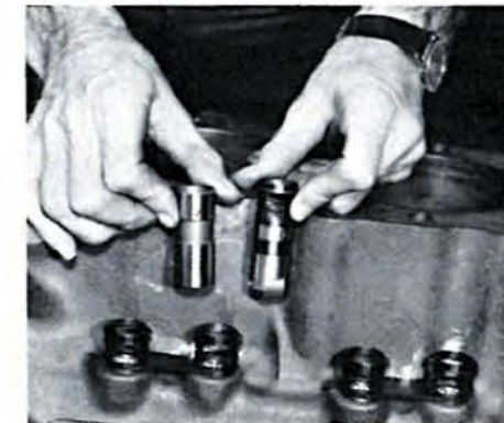
BELOW—Cam manufacturers offer solid, hydraulic, and roller lifters as part of the complete kit. The lifters are made to be compatible with the metals used in the cam itself.
