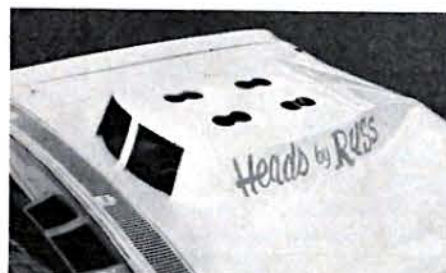
ABOVE—The Fenner Tubbs Plymouth is fitted with a zippered canvas bag that holds ice. When the ice melts, it passes through the fiber and trickles down across the entire radiator face. Then the water evaporates and carries off heat from the radiator. ABOVE RIGHT—Another idea for efficient cooling is hosing down the radiator face and keeping a towel on the top tank to hold water, release it during a run. This gasser runs without a fan, so other methods are needed. BELOW—Hood modifications, where allowed, will help. Holes in rear let hot air get out.
