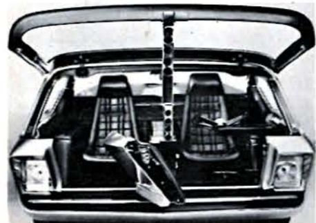
TOP OF PAGE—This is the "before" picture of a Dodge A-100 pickup truck as it was delivered to Detroit's Alexander Brothers. CENTER—The finished product of 2000 hours' labor is this low slung Dodge Deora custom, two feet longer and two feet lower than stock. The stock 6-cylinder engine was moved back 15 in., right to the middle of the bed, for cabin room. ABOVE—This front door really is one. Door is center-hinged, and window is hinged at top for easy entry into the plush cabin. The cut-down steering wheel connects to steering box via a bicycle chain enclosed in the swinging arm. While this truck is a showpiece, it has almost everything needed to drive on the street, including engine and transmission.
