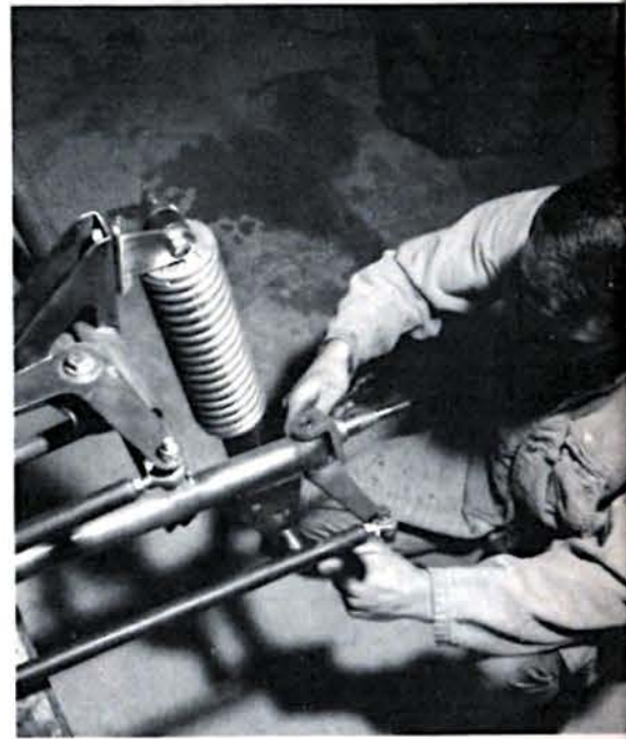
TOP OF PAGE, LEFT—Master welder Britting puts the finishing touches on a steering spindle flange before it's attached to the front axle assembly. LEFT—Finished front end shows Britting's treatment of coil-shock mounting, behind axle, with a sturdy top mount. ABOVE LEFT—Race Car Engineering's front end treatment is similar, using a longer spring and mounting it atop the axle. RCE has also built in six adjusting holes for spring height. ABOVE RIGHT—Another steering/suspension assembly, this time by Logghe Stamping Co. Unit fits behind axle and carries adjusting holes in mount plate.
