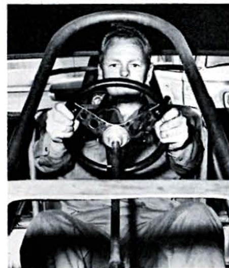
ABOVE —George Britting checks out the view from the bridge of a Dodge Charger funny. Cage protects driver in the event of a roll, and cut out area provides working room. RIGHT —Chassis technician uses heliarc welder on radius rod mounting bracket to provide strongest joint possible.
