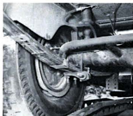
ABOVE LEFT—Rear suspension consists of leaf springs, vertical adjustable shocks, and adjustable traction bars. Tube member runs from side to side of axle housing in the rear. ABOVE—Another view of the rear end assembly, showing the reinforcing member, and the forward mounting plate for the short, stiff traction bars. LEFT—Springs and traction bars move in the same axis. Note the numerous reinforcing tubes and gusset plates in this portion of the tube frame. BELOW—"Tension II's" driver, Gary Bolger (l.), and owner/builder Bud Richter remove the glass hood panel to have a look at the engine.
