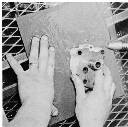
ABOVE—Proffitt checks the height of the wire ring above the block deck with a depth mike. RIGHT—To increase oil pump capacity, get a glass plate and a large sheet of 400 wet-or-dry sandpaper, run pump body and end plate over paper to decrease clearance, up output. BELOW—Finished O-ring job looks like this. Note super sano block.
