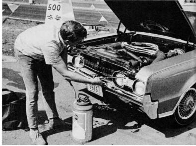
tire top surface of the engine was packed in ice, the intake tubes were sprayed down, and the radiator core doused with water. Timing was slipped back to original 13° setting.
