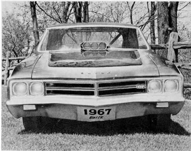
ABOVE LEFT—Head-on view of Ron Pellegrini's Buick Gran Sport hardtop reveals a lot to the trained eye, such as the fiberglass bodywork, Dzus fasteners, and a bugcatcher coming through the windshield. ABOVE RIGHT—On the other end, there's still more fiberglass, wheelie bars, Simpson 16-ft. parachute, and a set of Goodyear 1100 x 16 slicks. One gets the impression that all that glitters is not stock Buick.
