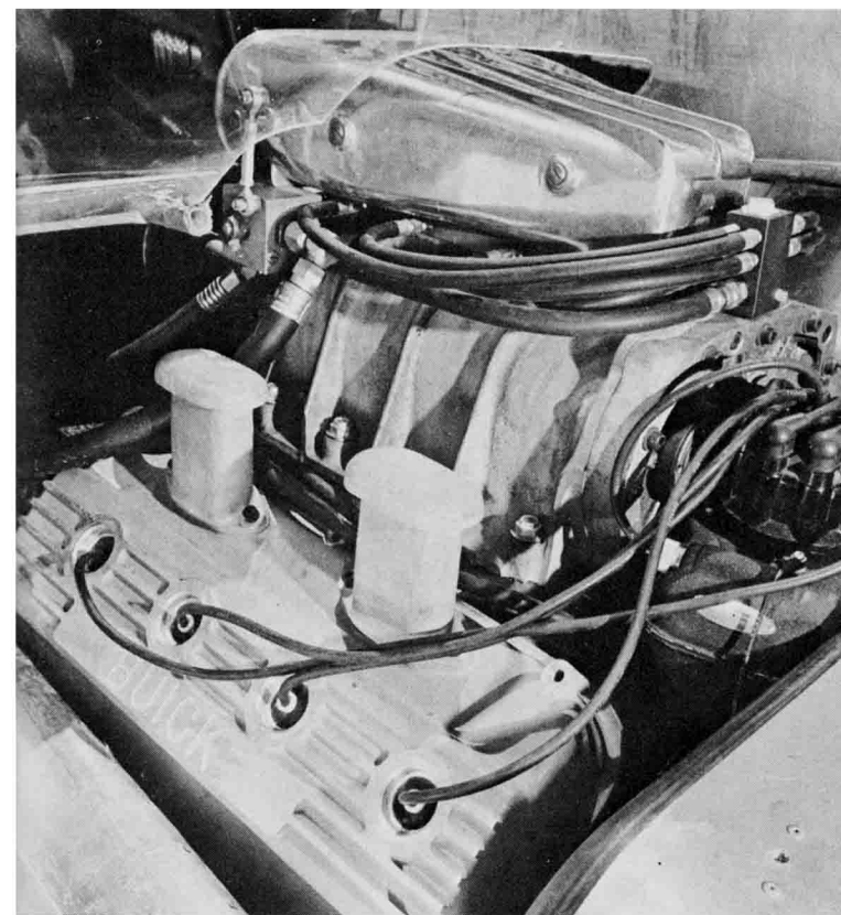
ABOVE—Here's the clincher. It's a 430-in. MoPar hemi, carrying MIT pistons, rods, and rings, Milodon main support, Crane cam, Donovan rockers, valves, and covers, Enderle injector, Schiefer magneto, and heads by DuPage Automotive. The 6-71 huffer is driven by a Cragar/Thompson drive, and sits on a Cragar manifold. Overdrive is 20%. TOP RIGHT—Interior aluminum is .032 sheet, formed by the owner, supported by the NASCAR roll cage, and supporting a Corvair steering unit. ABOVE RIGHT—Neat headers are by Rudy's Custom Exhaust, of Cicero, Ill. Direct drive by Henry Machine uses Schiefer plate, Velvetouch disc, and a Donovan wheel. RIGHT—Rear features vertical Delco airshocks, NASCAR leaves, much bracing, and stiffening members added to chassis.
