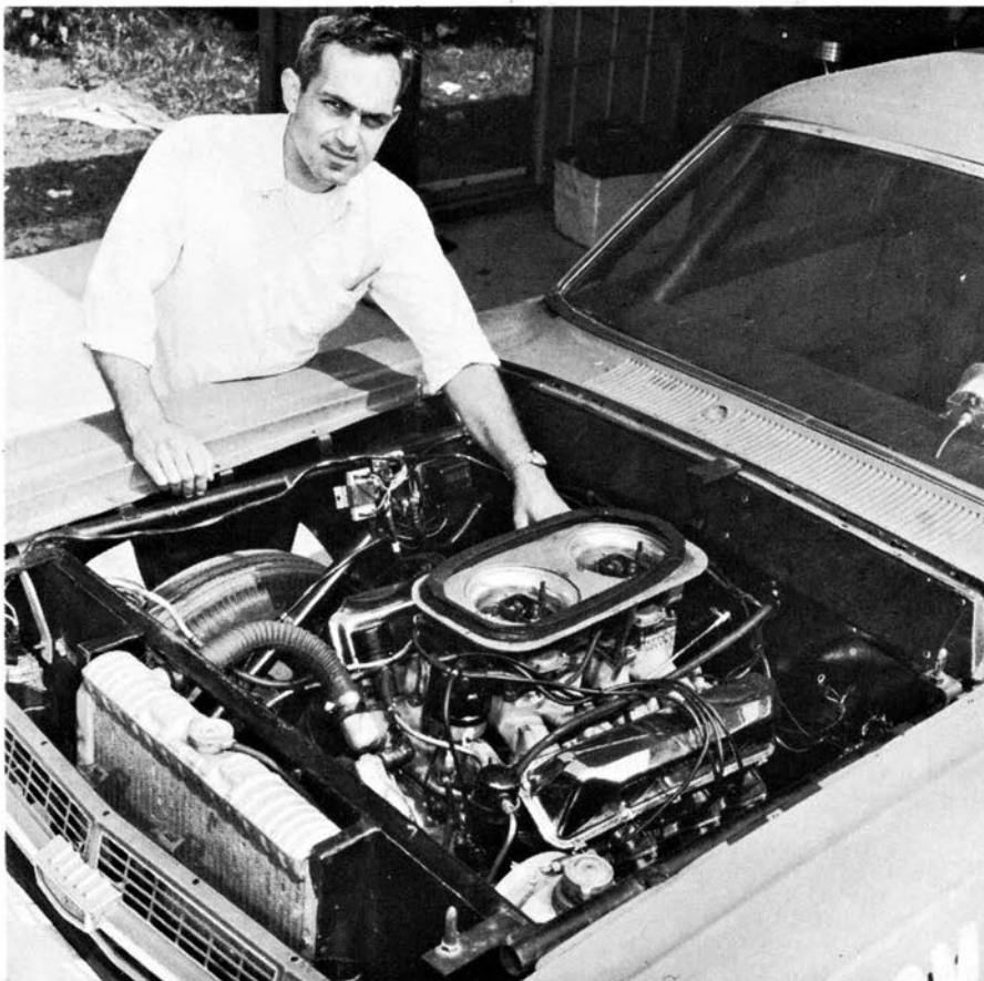
Left, Dave Lyall with his Tunnel Port 427 wedge. Engine pulls well past the point where straight wedges die. Above, ports are large enough to swallow intake valve.
