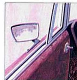
**Remote-Control Outside Rearview Mirror.** Provides clear view of approaching traffic and makes it easy to set the mirror at the most desirable angle. Without lowering the window, you can quickly aim the mirror by simply moving the inside fingertip control.
