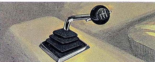
**4-Speed Manual Transmission** . . . Sports-type, close-ratio 4-speed manual transmission is available on sedans and coupes with either of the V-8's. Fully synchronized. Positive reverse gear lockout. Familiar floor-mounted stick shift.
