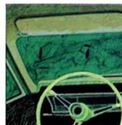
**Thick-Laminate Safety Plate Glass Windshield** offers greater strength and protection. New Padded Windshield Pillars on either side. Padded Sun Visors overhead and Padded Instrument Panel, combine to provide added protection for the driver and front seat passengers.
