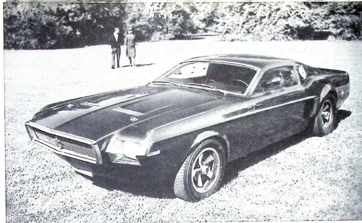
Don't rush down to your neighborhood Mustang dealer—quite yet. The Mach 1 is only an experimental model, but these "dream" show cars often portend the future. Reflecting Ford GT styling, the quick-release fuel filler caps behind the fixed sideglass, functional rear brake air intakes, and the 64-degree raked windshield stress the accent on "sports" in this sports-personal car direction for styling.
