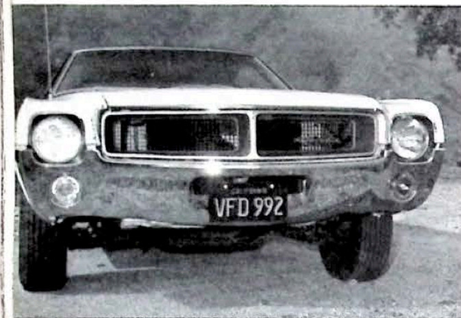
Javelin plastic grille means less chance of rust in this vulnerable area, and is lightweight. Wraparound bumper protects sheetmetal and lights, but costs more to replace. Flow-through vent exit point is beneath large armrest. Good looking flush outside door release brightens looks, and is a snap to operate.
