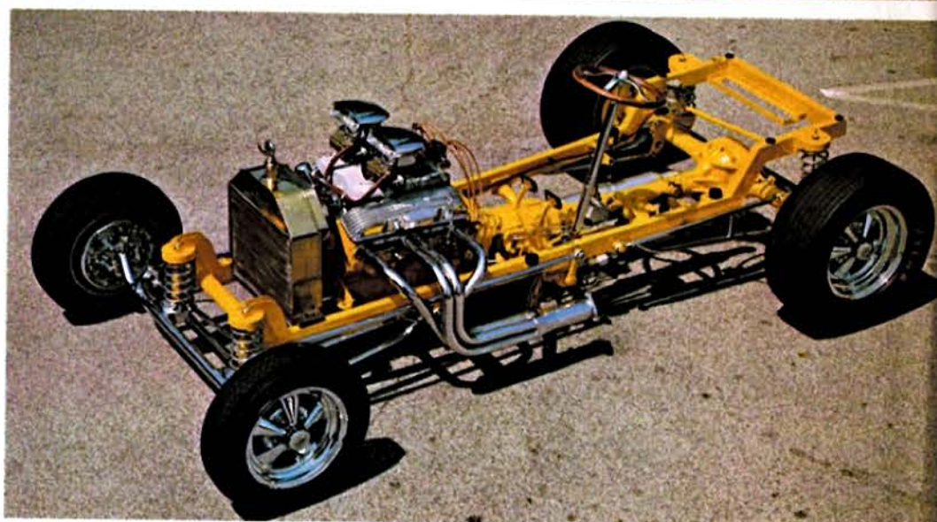
All finished and ready for tour, builder Dick Scritchfield takes spin in street rod. Body is Cal Automotive's fiberglass replica of 1923-T behind a '67 327 Chevrolet engine and "new" 1915 radiator. First of its kind to feature coil spring suspension. Wheels are Cragar S/S mounting Goodyear Sports Car Specials.
