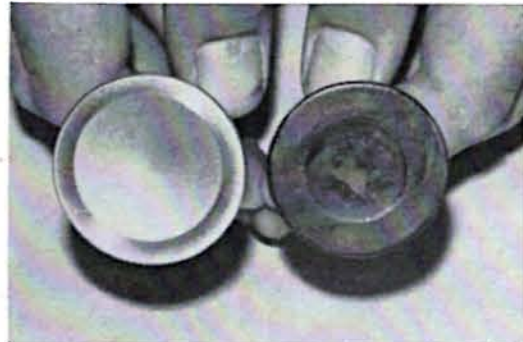
ABOVE — The stock 1 1/2-inch Chevrolet exhaust valves, on right, are discarded and replaced with a new set of hard-chromed 1 1/4-inch valves.
