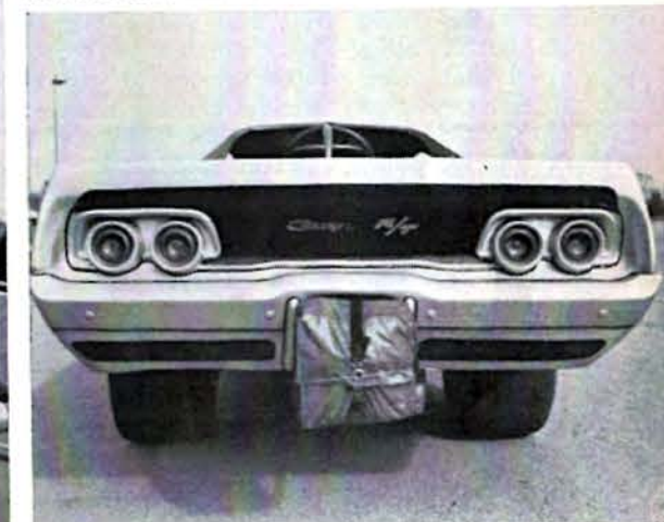
BELOW & BOTTOM — Although both pictures are of the same finished product, a little trick camera work by CAR CRAFT's staff photog shows the difference achieved when the 10-inch section is removed from body.
