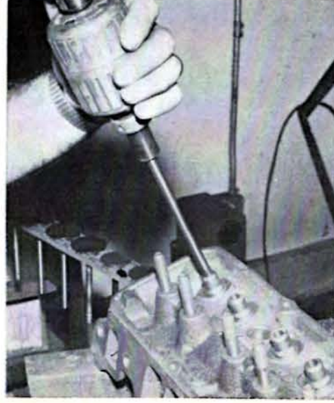
ABOVE — Talk about slick ports, these numbers almost have the Grand Canyon beat! Mondello's porting treatment of the exhausts was accomplished with carbide burrs and resin cloth.
