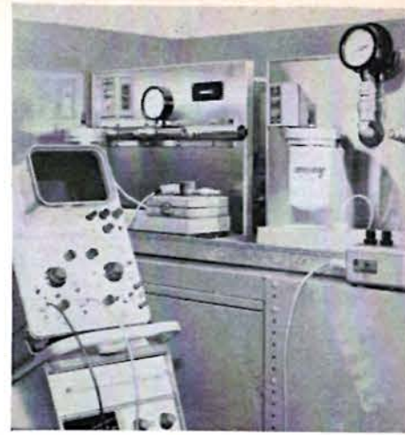
Exhaustive testing lies behind all racing filter design features. Here a filter undergoes surge testing to evaluate its ability to withstand fatigue failure because of internal cyclic pressure changes.
