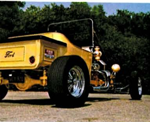
All finished and ready for tour, builder Dick Scritchfield takes spin in street rod. Body is Cal Automotive's fiberglass replica of 1923-T behind a '67 327 Chevrolet engine and "new" 1915 radiator. First of its kind to feature coil spring suspension. Wheels are Cragar S/S mounting Goodyear Sports Car Specials.
