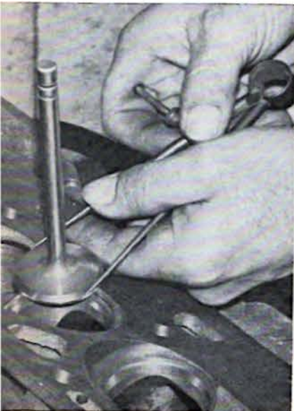
ABOVE — The stock 1 1/2-inch Chevrolet exhaust valves, on right, are discarded and replaced with a new set of hard-chromed 1 1/4-inch valves.
