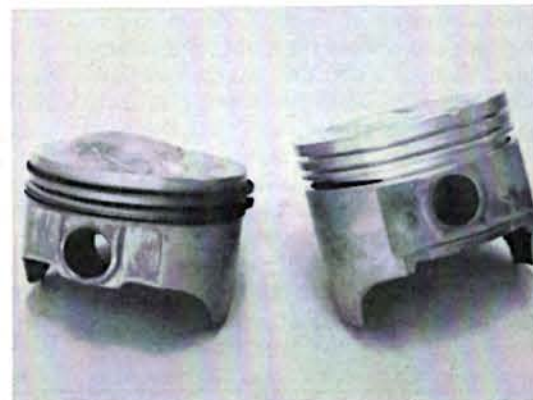
ABOVE — The standard 302 engine uses the flat top piston for 10.5:1 compression, while the high performance mill uses pop-ups for 12.5:1 ratio.
