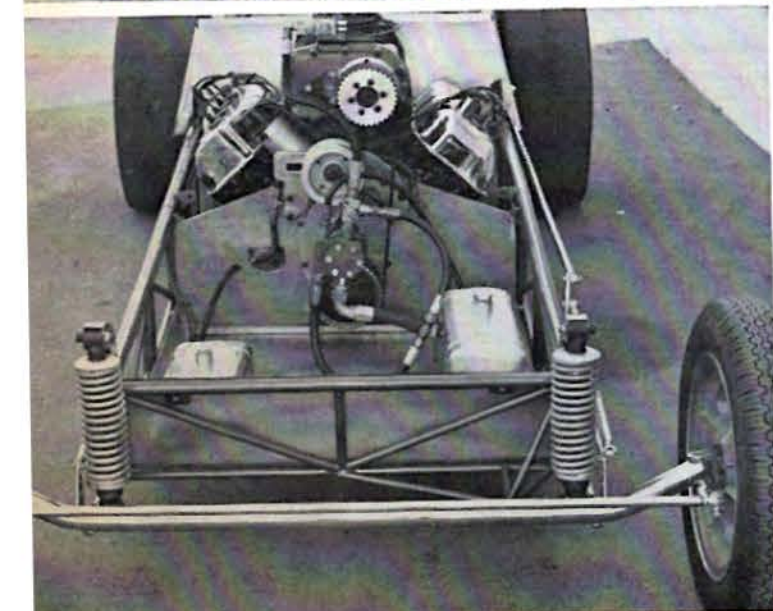
ABOVE — In early construction phases, the "funny" almost resembled a dragster, with rear-mounted driver's position and dragster-like cage. The 128-inch wheelbase adds to the "new look" in chassis technique.
