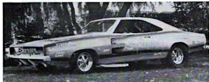
First '68 "funny" to emerge was Don Schumacher's "Stardust." Injected Illinois Dodge has Fiber Glass Ltd. Charger body.
