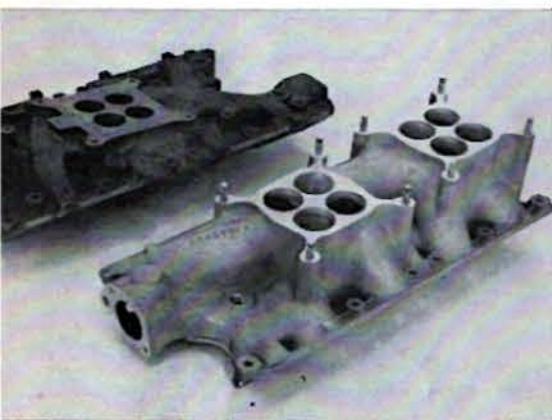
ABOVE — Essentially, the combustion chambers of the 302 resemble those of their brother, the 289. One exception is valve sizes, 2.15 intakes and 1.56 exhausts. LEFT — How much carburetion do you want? There is a choice between a single four or dual four-barrel manifold for the standard and high performance 302.
