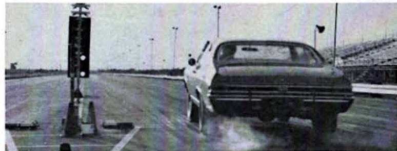
ABOVE — Casler slicks did great job of launching 396's 375 horses off the line, but 3.08 "bog" gear pulled rpm way down just off line. RIGHT — Full power was delivered after disconnecting smog devices (visible above headers) and installing a set of tubular Hooker headers.
