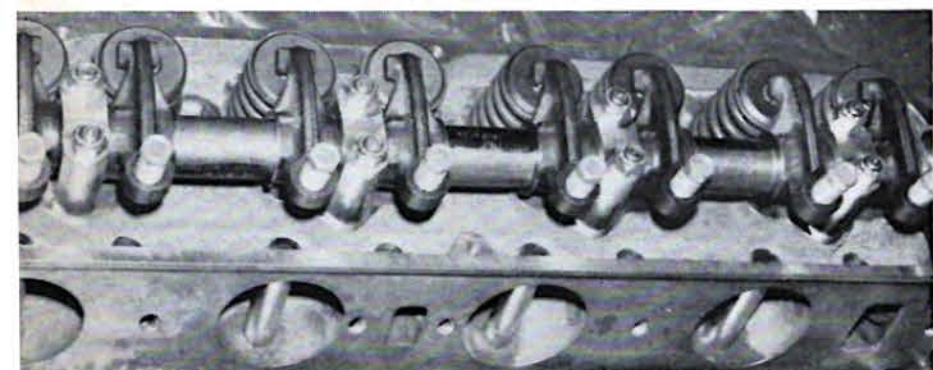
BELOW — This is her! Giant 2.20-inch tunnel ports with push rod sleeve are a duplicate of big 427-type heads. That hardened hollow alloy steel rocker shaft allows adjustment and high rpm operation.
