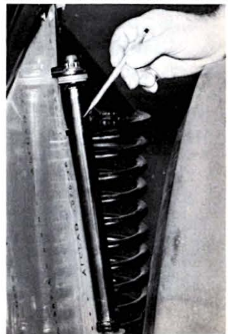
BELOW — Joe's gold pencil points out key to car's split personality rear suspension. Setup allows strip-side change.
