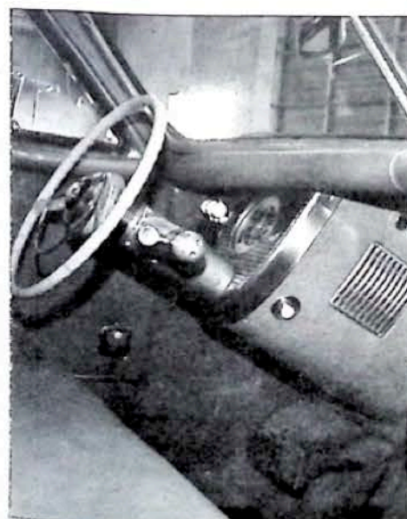
This '48 Tucker prototype has padded dash, pop-out windshield, breakaway mirror, knobless dash, "crash compartment."
