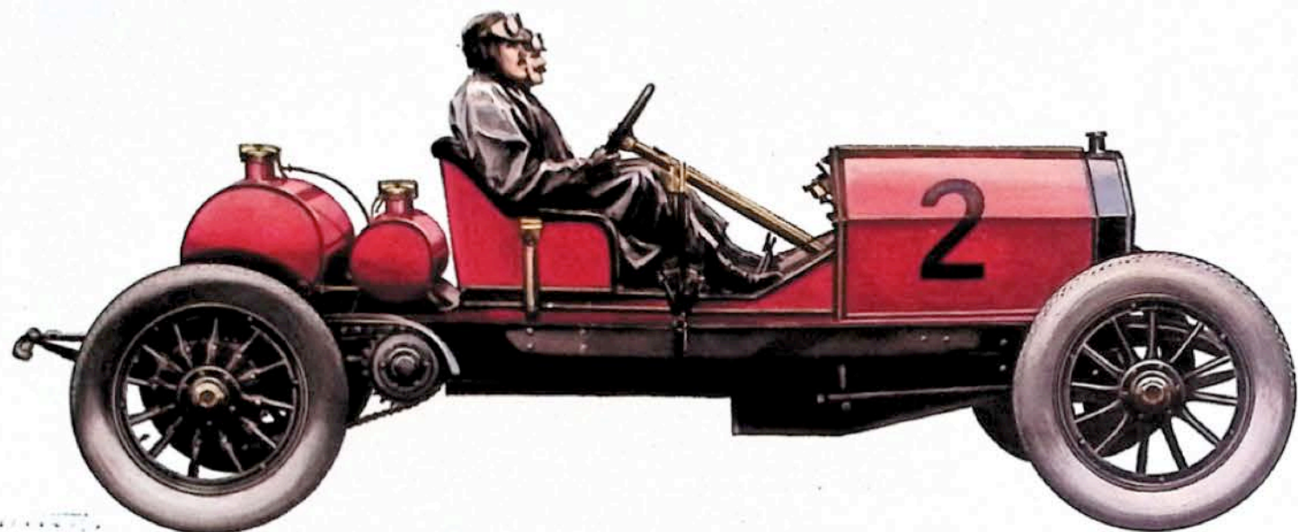
The 50-hp Simplex "Speed Car" is as much coveted by collectors as its contemporary, the Mercer "Raceabout." In its heyday, the Simplex cost more than twice as much as the Mercer — about $6000. The two tanks behind the seats are for gasoline and oil. The oil — 13 gallons of it — is in the smaller of the two tanks.
