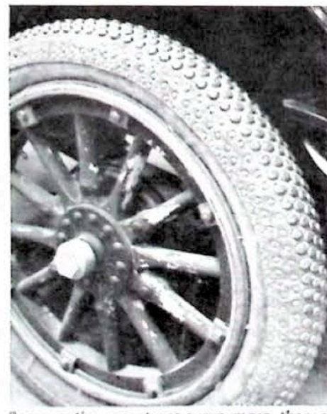
Because tire punctures were more than a nuisance in 1912, many motorists installed these steel-studded leather tire boots.
