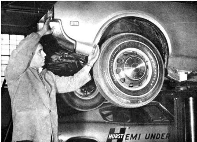
LEFT—Front overhang on 442 is almost two inches less than overhang of big Toronado. BELOW LEFT—The 3½-inch Toronado tube axle was retained, but suspension had to be altered to provide better braking action. Oddball shock setup from Toronado was changed. RIGHT—Rear coil springs are the lightest-duty units available, but they work well with altered suspension pivot points. BELOW—Cornering, acceleration, and turning were improved vastly.
