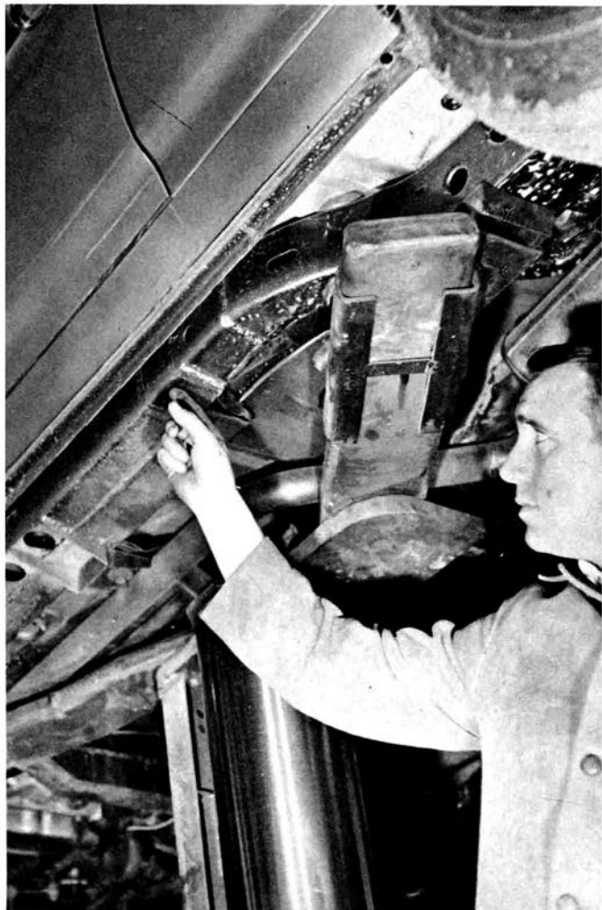
ABOVE LEFT—The project started with a Toronado chassis, which was modified front and rear to mate with the 442 body, but retained drive system layout. ABOVE—Conversion altered front of Toronado frame enough to get 442 body and bumpers to fit, and the end result was an increase in wheelbase of 2.5 inches to 114.5 inches. LEFT—Dave Landrith, Hurst Detroit engineer, is the guy who thought up the project. Here he shows the spot where Toronado frame (front) joins 442 frame. BELOW—At the extreme front of the engine room, some of the sheet metal had to be trimmed away to make the radiator fit in right.
