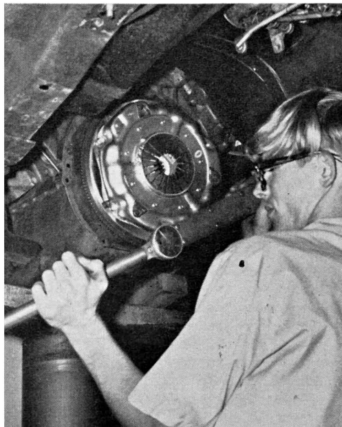
ABOVE — Mike Edgar of the Pharaoh's Pacers car club carefully checks installation of the clutch with a torque wrench, a must to do the job right. 'Pacers are sponsored by Dick Allen Rambler, pioneer in fast-growing Rambler car club activities.
