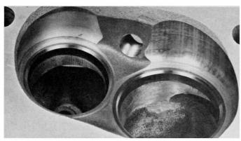
Normally a chamber volume of 109.6 cc's is correct, but to compensate for carbon buildup which occurs on the street. go to a corrected volume of 107.5 cc's.
