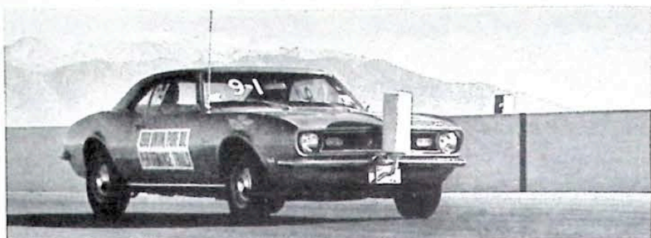
Economy phase of the trials was revised for 1968. Insulated container of fuel cooled to specified temperature was attached to front of car and mpg computed from fuel consumed.
