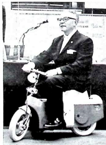
Michael Yardney demonstrates an English mini-scooter powered by his company's economical Zynoxel zinc-air battery.
