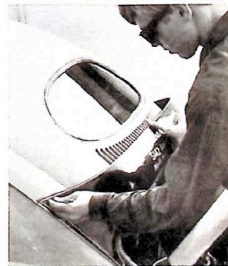
The Volkswagen Super Scoop is a fiberglass air scoop that is attached over intake vent holes. It uses the air stream to produce a ram effect into the engine area for cooler oil temperature. Purveyors of Super Scoop also claim it serves as a spoiler.
