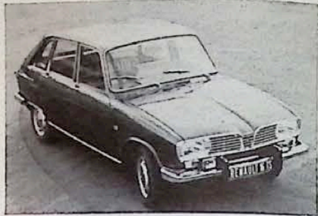
(Top) Recent sensation de Tomaso Mangusta by Ghia is now emphasized by roadster. (Above) Renault has a new R16 T.S. for the sporty minded. With 1600cc and 92 hp, the car will now do 100 mph, 0 to 50 in 8 seconds, 0 to 60 in only 13 seconds.
